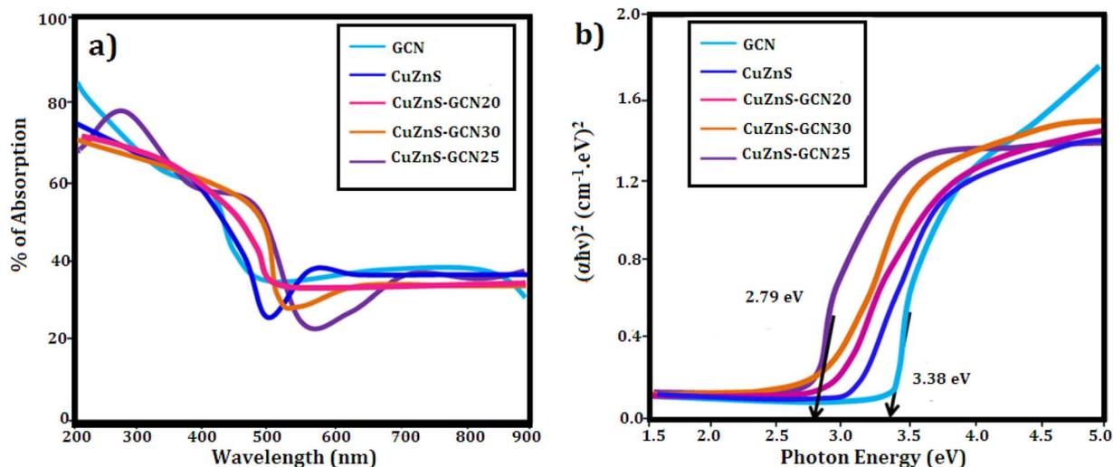
Fig. 4 (a) UV-DRS spectra of g-C<sub>3</sub>N<sub>4</sub>, CuZnS, CuZnS-GCN20, CuZnS-GCN25 and CuZnS-GCN30 samples. (b) Tauc plot of band gap calculation.
