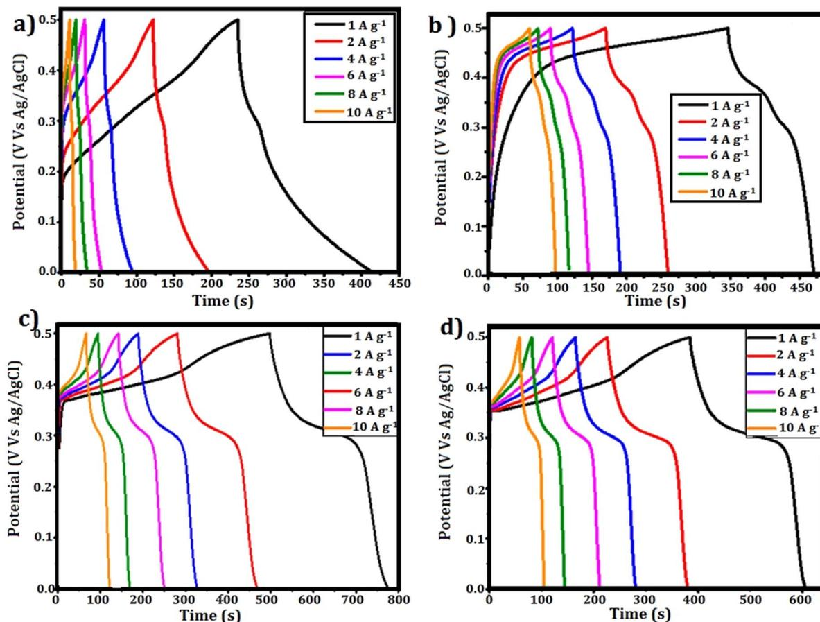
Fig. 9 GCD curves of (a) CuZnS (b) CuZnS-GCN20 (c) CuZnS-GCN25 and (d) CuZnS-GCN30 electrodes at various current densities.
