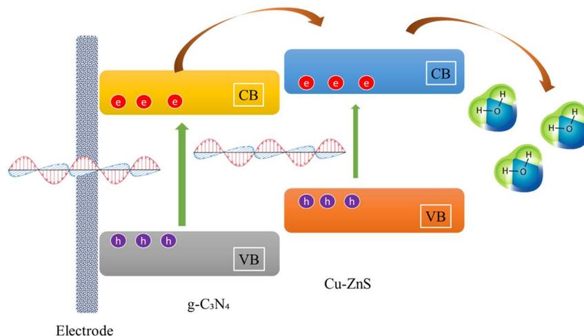
Fig. 14 A schematic energy band diagram showing the charge transfer between Cu-ZnS and g-C<sub>3</sub>N<sub>4</sub> and photocatalytic mechanisms.
