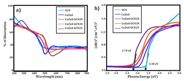
Fig. 4 (a) UV-DRS spectra of g-C<sub>7</sub>N<sub>4</sub>, CuZnS, CuZnS-GCN20, CuZnS-GCN25 and CuZnS-GCN30 samples. (b) Tauc plot of band gap calculation.
