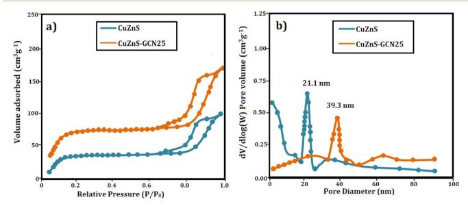
Fig. 5 (a)  $N_2$  adsorption—desorption isotherm of CuZnS and CuZnS-GCN25 (b) BJH plot for pore size calculation.
