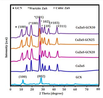
Fig. 1 Powder XRD patterns of the prepared samples.
