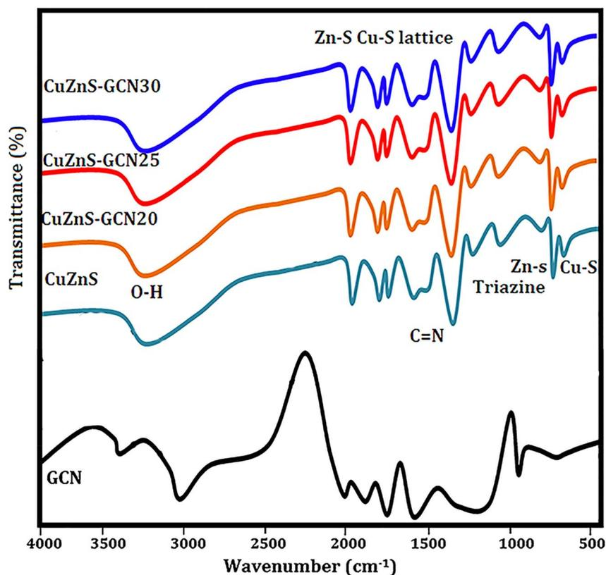
Fig. 3 FTIR spectra of the prepared samples.
