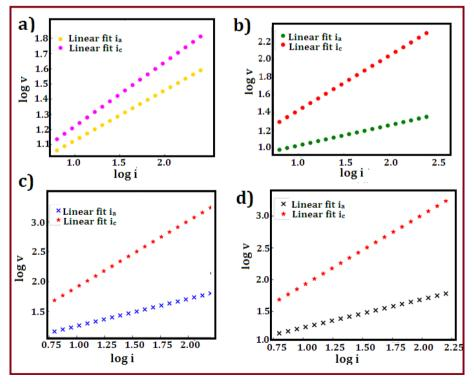
Fig. 8 Logarithmic plot of peak current (/p) vs. scan rate (v) for (a) CuZnS, (b) CuZnS-GCN20, (c) CuZnS-GCN25 and (d) CuZnS-GCN30 electrodes.
