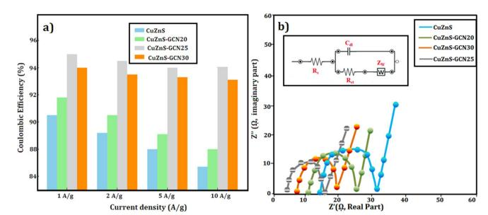
Fig. 10 (a) Coulombic efficiency (%) vs. current density (b) Nyquist plot.
