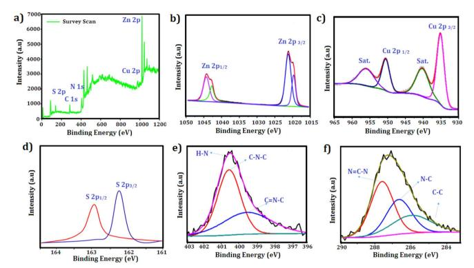
Fig. 6 XPS spectra results of CuZnS-GCN25 (a) survey scan spectra; core level scan (b) Zn 2p (c) Cu 2p (d) S 2p (e) N 1s (f) C 1s.
