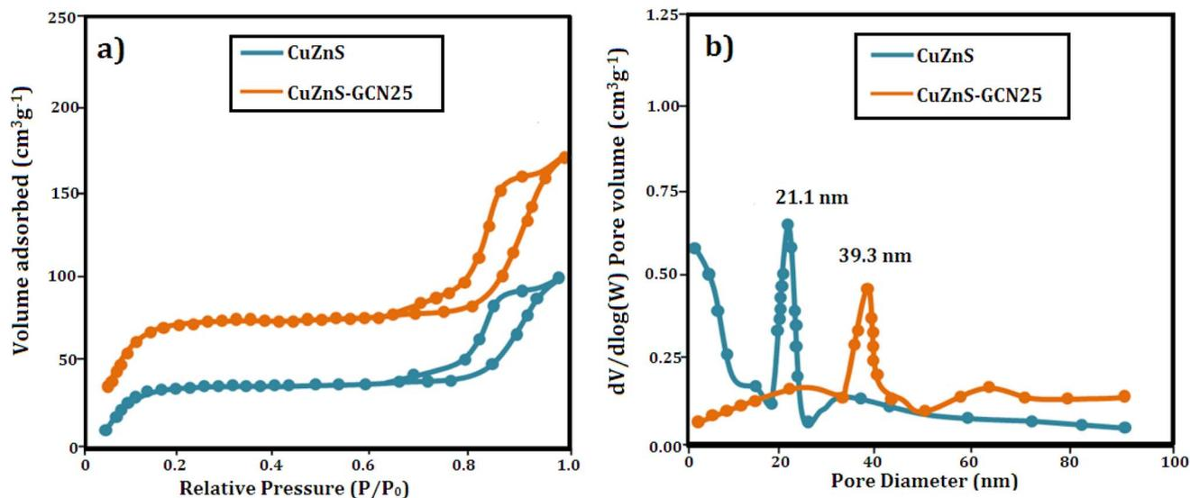
Fig. 5 (a) N<sub>2</sub> adsorption–desorption isotherm of CuZnS and CuZnS-GCN25 (b) BJH plot for pore size calculation.
