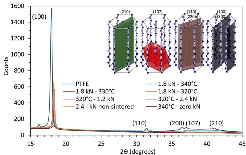
Fig. 3 XRD diffractograms of the prepared samples.
