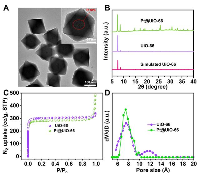
Fig. 1 (A) TEM images of Pt@UiO-66. (B) PXRD patterns of UiO-66 and Pt@UiO-66. (C) N<sub>2</sub> adsorption–desorption isotherms at 77 K of UiO-66 and Pt@UiO-66. (D) Pore size distributions of UiO-66 and Pt@UiO-66.
