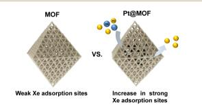
**Scheme 1** Encapsulation of Pt NPs with strong Xe adsorption sites in a MOF to enhance Xe/Kr separation.
