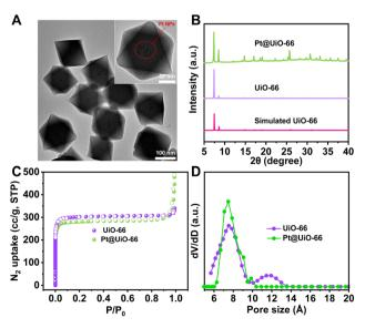
Fig. 1 (A) TEM images of Pt@UiO-66. (B) PXRD patterns of UiO-66 and Pt@UiO-66. (C)  $N_2$  adsorption—desorption isotherms at 77 K of UiO-66 and Pt@UiO-66. (D) Pore size distributions of UiO-66 and Pt@UiO-66.
