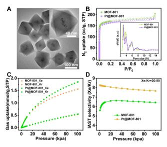
Fig. 4 (A) TEM images of Pt@MOF-801. (B)  $N_2$  adsorption—desorption isotherms at 77 K and pore size distributions of MOF-801 and Pt@MOF-801. (C) Kr and Xe adsorption isotherms at 298 K of MOF-801 and Pt@MOF-801. (D) Calculated IAST selectivity for a Xe/Kr mixture (v/ v=20/80) for MOF-801 and Pt@MOF-801 at 298 K.
