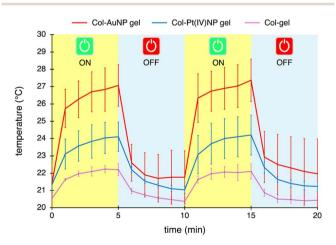
Fig. 3 Time course plots of temperature fluctuation under Yb:YAG green laser irradiation (515 nm). The error bars mean the standard deviations calculated from four independent experiments.
