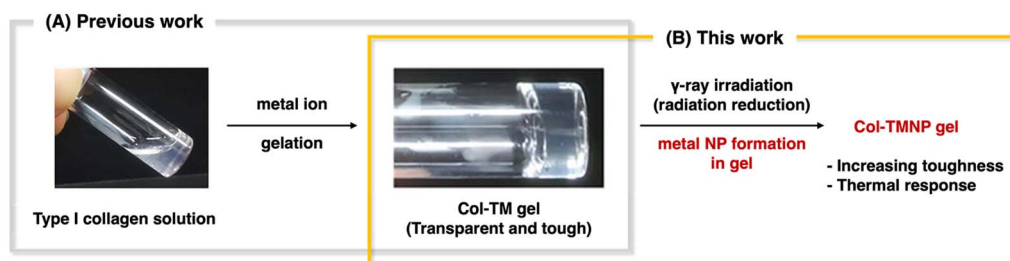
Scheme 1 \gamma -ray radiation induced metal nanoparticle formation in collagen gel. (A) Previous work. (B) This work.
