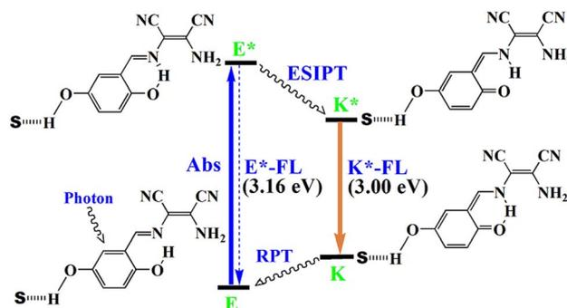
Fig. 3 Fluorescence emission mechanisms of **H<sub>2</sub>L** via ESIPT; S = DMF, EtOH or MeCN.
