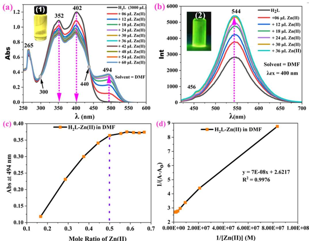
Fig. 4 UV-vis absorbance spectra (a), FL emission spectra (b), Job's plot (c), and Benesi–Hildebrand plot (d) of  $\text{H}_2\text{L}$  with Zn(II) in DMF. Insets show the color changes of  $\text{H}_2\text{L}$  upon Zn(II) addition under natural light (1) and UV light (2).
