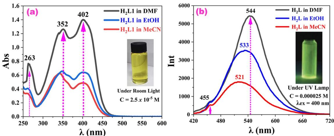
Fig. 2 UV-vis absorbance (a) and FL emission (b) spectra of **H<sub>2</sub>L** in different solvents.
