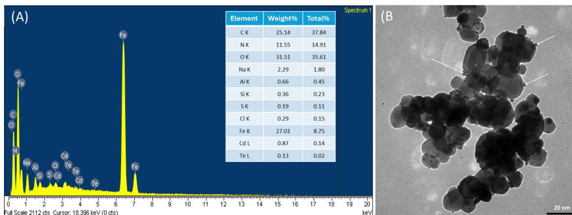
Fig. 2 EDX spectrum (A) and TEM image (B) of C3 NPs.
