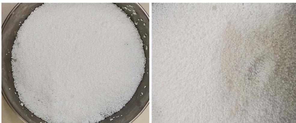
Fig. 9 Struvite pellet images from the FBHC process.
