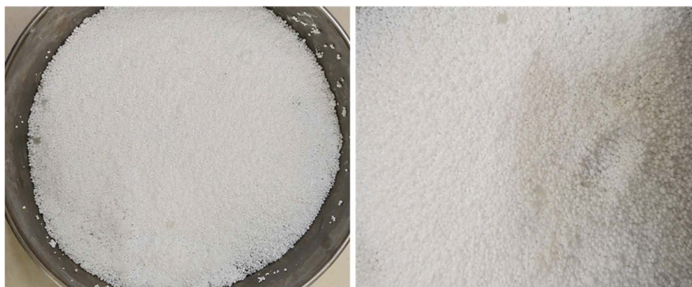
Fig. 9 Struvite pellet images from the FBHC process.
