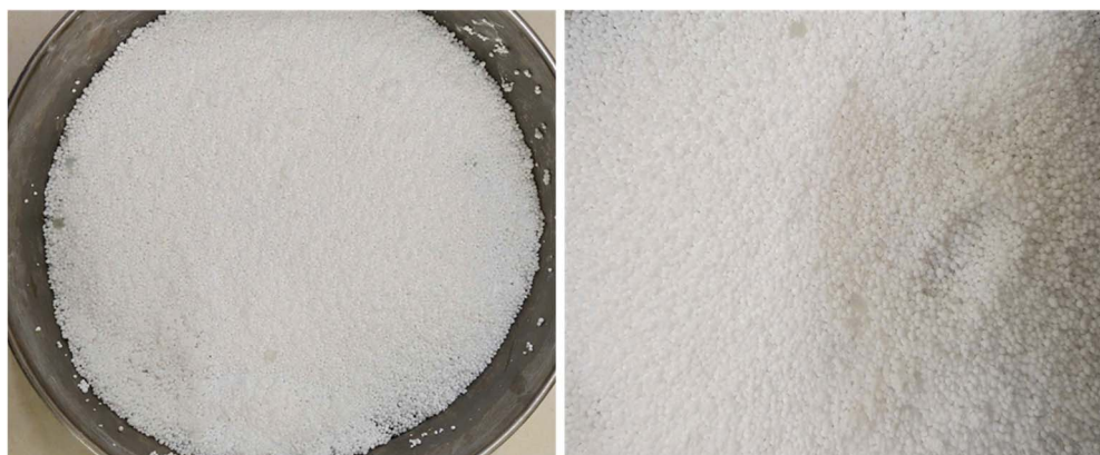
Fig. 9 Struvite pellet images from the FBHC process.
