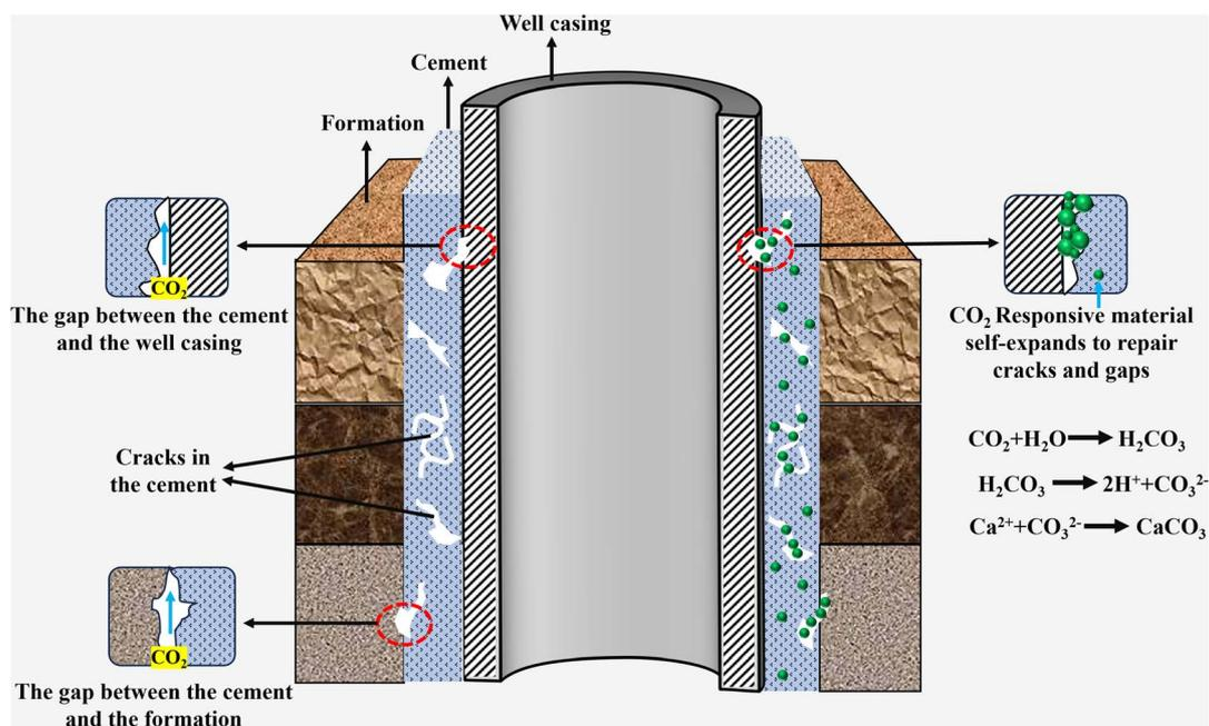
Fig. 5 Application of CO<sub>2</sub> responsive materials in cementing operations.
