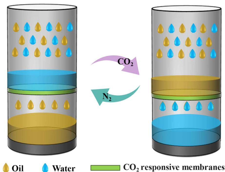
Fig. 8 Schematic diagram of oil–water separation regulated by CO<sub>2</sub> responsive membrane.
