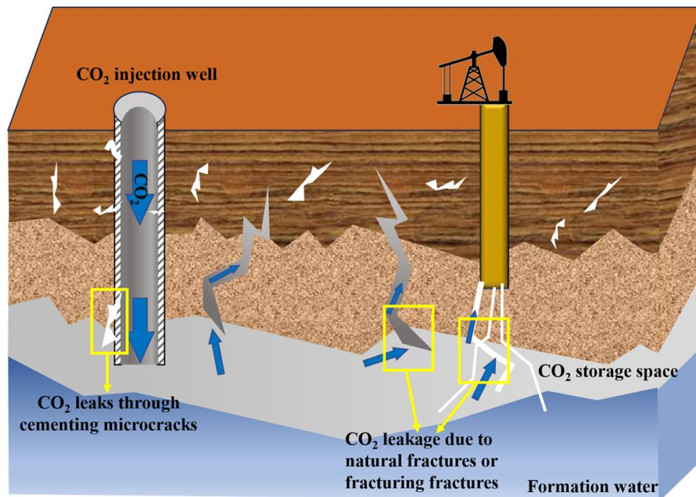
Fig. 13 Schematic diagram of CO<sub>2</sub> leakage during geological burial of CO<sub>2</sub>.
