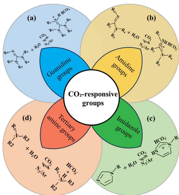
Fig. 3 Reversible response mechanism of CO<sub>2</sub> responsive functional groups.
