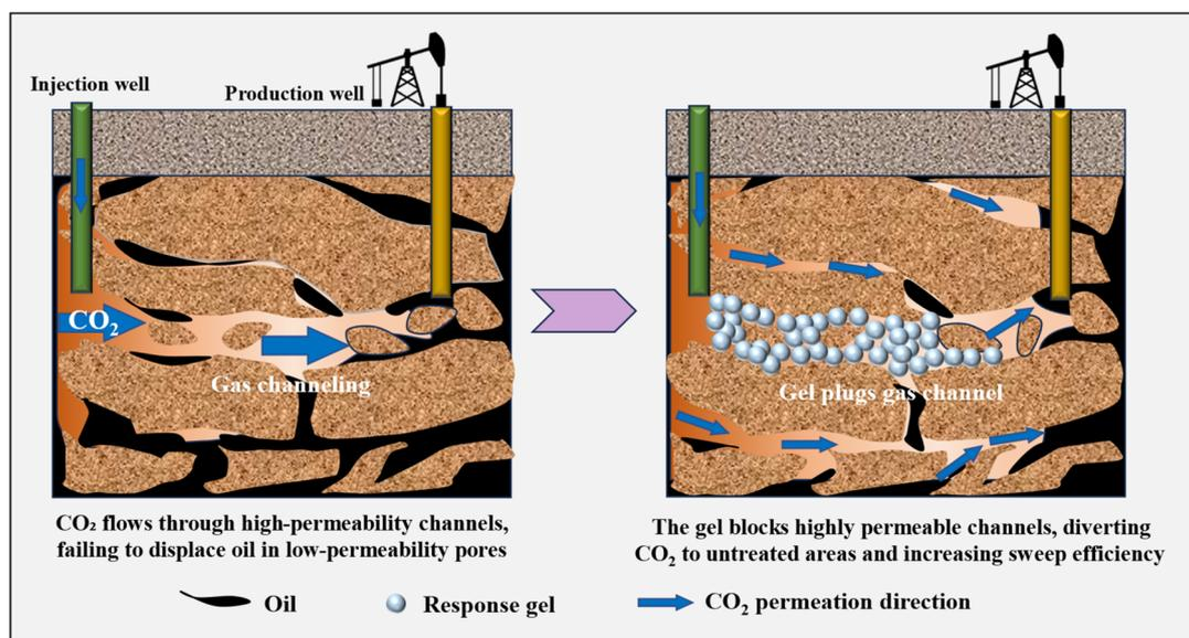
Fig. 11 Schematic diagram of CO<sub>2</sub> responsive gel plugging gas channel for enhanced oil recovery.
