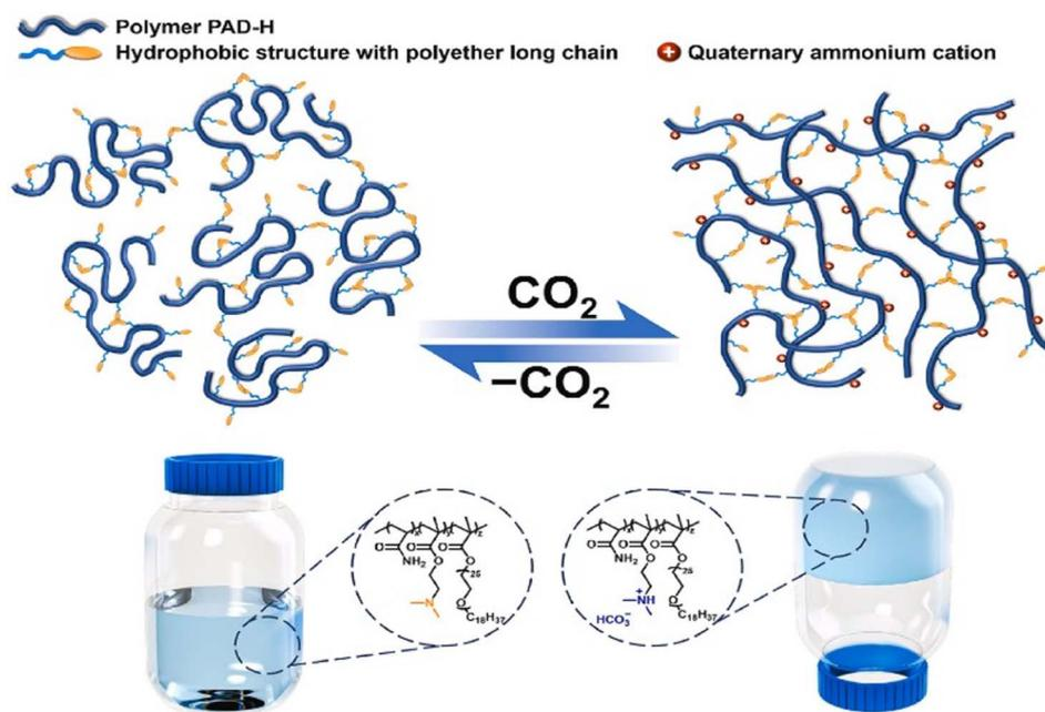
Fig. 10 Schematic diagram of CO<sub>2</sub> responsive viscosity-increasing mechanism of PAD-H. This figure has been reproduced from ref. 106 permission from Elsevier, copyright (2024).
