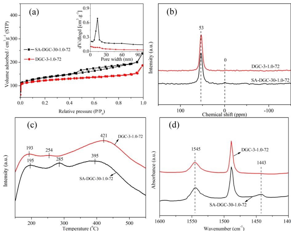
Fig. 5 (a) N<sub>2</sub> adsorption–desorption isotherms and BJH mesopore size distribution, (b) <sup>27</sup>Al MAS NMR spectra, (c) NH<sub>3</sub>-TPD curves and (d) FT-IR spectra of adsorbed pyridine of SA-DGC-30-1.0-72 and DGC-3-1.0-72.
