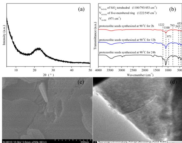
Fig. 1 (a) XRD pattern of protozeolite seeds synthesized at 90  $^{\circ}\text{C}$  for 24 h. (b) FT-IR spectra of protozeolite seeds synthesized at 90  $^{\circ}\text{C}$  and at different times. (c) SEM and (d) TEM images of protozeolite seeds synthesized at 90  $^{\circ}\text{C}$  for 24 h.
