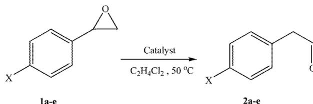
Scheme 1 Rearrangement of 4-substituted styrene oxides (1a–e).
