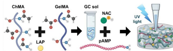
Fig. 1 Schematic representation of the hydrogel synthesis. Methacrylated chitosan (ChMA) and methacrylated gelatin (GelMA) were combined with the photoinitiator LAP to form the GC precursor solution. N -Acetylcysteine (NAC) and pro-adrenomedullin peptide (PAMP) were added before photopolymerization under UV light to obtain the final crosslinked hydrogel.
