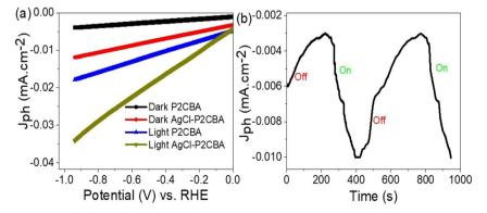
Fig. 4 (a) The PEC response of the fabricated P2CBA and AgCl-P2CBA for H<sub>2</sub> gas generation from splitting Red Sea water under white light (b) on/off chopped light for AgCl-P2CBA composite electrode.
