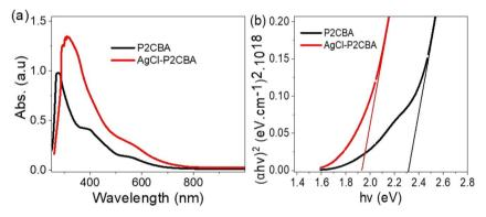
Fig. 3 (a) Optical absorbance (b) Tauc spectra of P2CBA polymer and AgCl-P2CBA nanocomposite.
