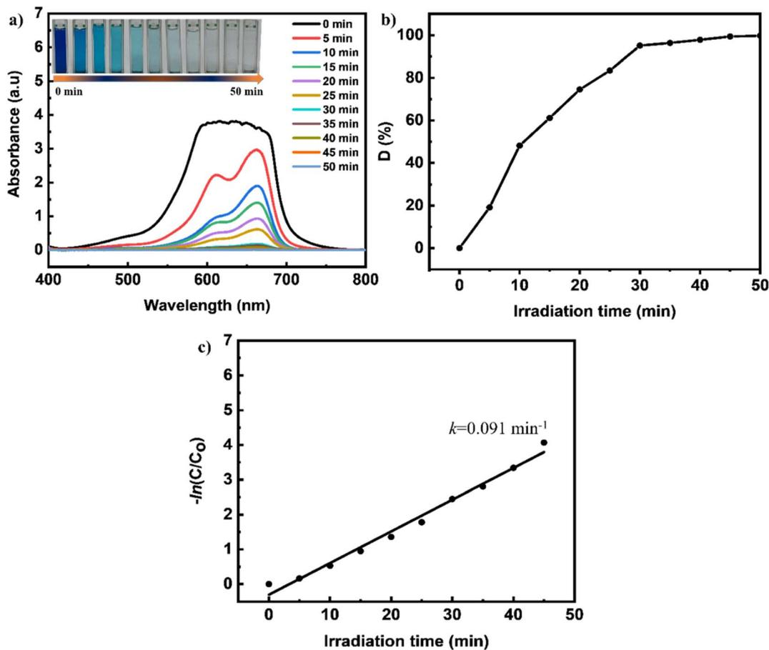
Fig. 7 (a) Time-dependent UV-vis absorption spectra of  $10^{-4}$  M MB degradation in the presence of C-TiO<sub>2</sub>-MoS<sub>2</sub> under visible light, (b) MB degradation percentage and (c) degradation rate, respectively.
