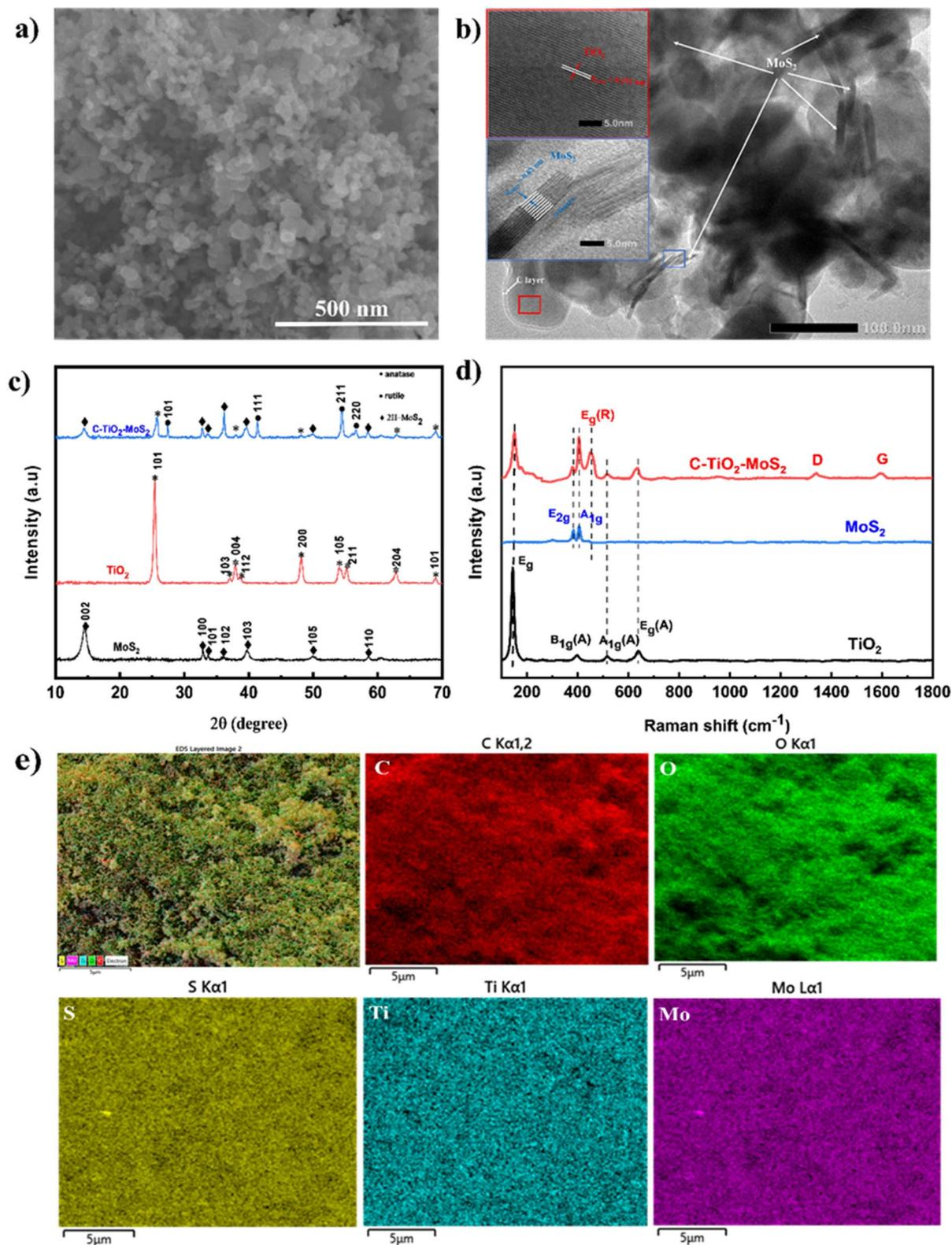
Fig. 2 (a) SEM, (b) HRTEM image, (c) XRD pattern, (d) Raman spectra, and (e) EDS elemental mapping of C-TiO<sub>2</sub>-MoS<sub>2</sub> nanocomposite.
