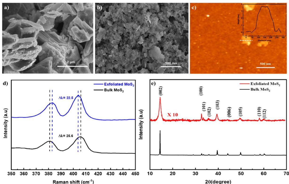
Fig. 1 (a) SEM image of bulk MoS<sub>2</sub>, (b) SEM image of as-exfoliated MoS<sub>2</sub> nanosheets, (c–e) AFM image, Raman spectra, and XRD patterns of bulk MoS<sub>2</sub> and as-exfoliated MoS<sub>2</sub>. Inset is the height profile of as-exfoliated MoS<sub>2</sub> in (c).
