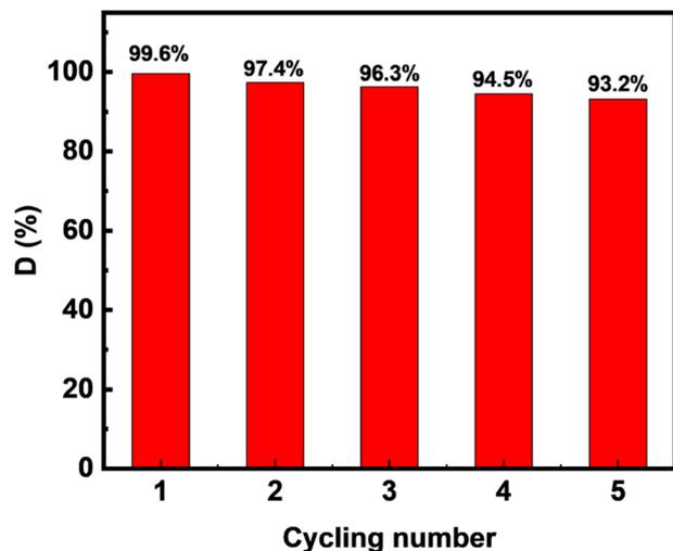
Fig. 4 Five consecutive cycles for the MB photodegradation using C-TiO<sub>2</sub>-MoS<sub>2</sub> nanocomposite.
