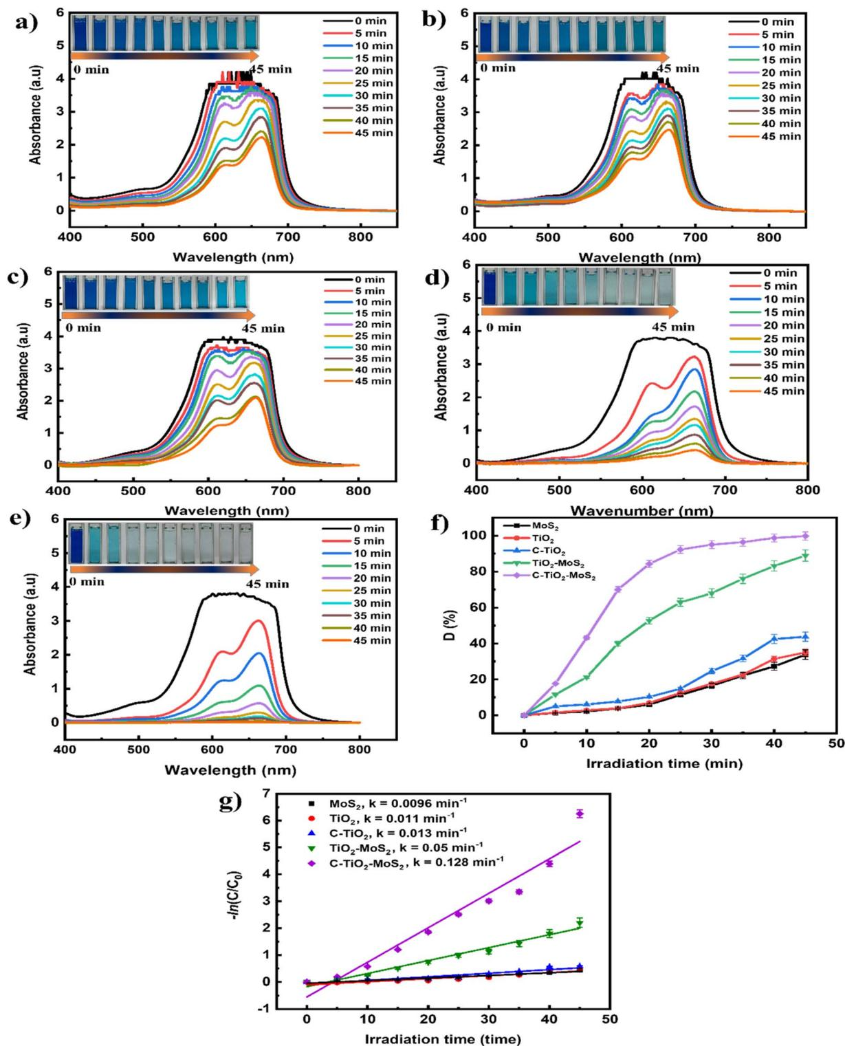
Fig. 3 Time-dependent UV-vis absorption spectra of MB ( $10^{-4}$  M) degradation in the presence of (a) bare TiO<sub>2</sub>, (b) bare MoS<sub>2</sub>, (c) C-TiO<sub>2</sub>, (d) TiO<sub>2</sub>-MoS<sub>2</sub> and (e) C-TiO<sub>2</sub>-MoS<sub>2</sub> under UV irradiation. (f) and (g) are MB degradation percentage and degradation rate of the samples, respectively.
