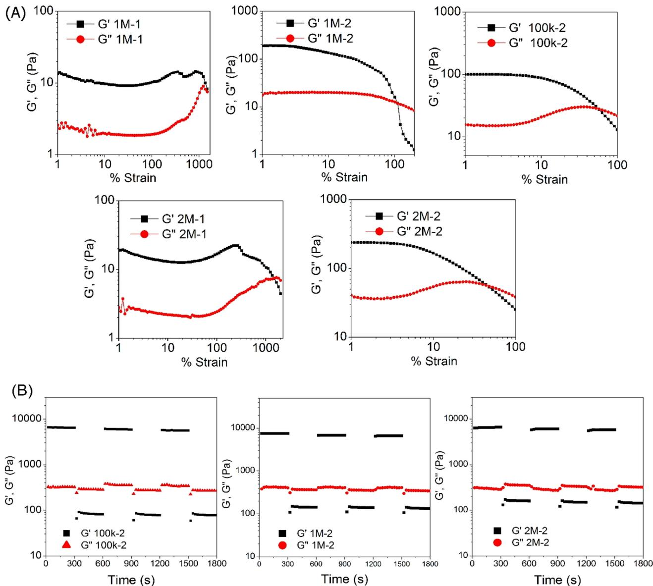
Fig. 6 The rheological studies of hydrogels: (A) strain sweep of hydrogels 1M-1, 1M-2, 2M-1, 2M-2, and 100k-2 at 37 °C. (B) Alternate step strain switch from 1% and 150% strain of 100k-2, 1M-2, and 2M-2 hydrogels.
