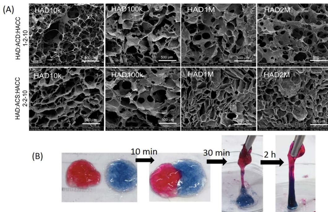
**Fig. 4** The morphology of hydrogels. (A) SEM images of hydrogels (10k-1, 100k-1, 1M-1, 2M-1, 10k-2, 100k-2, 1M-2 and 2M-2 respectively); (B) visual observation of hydrogel formation for 100k-2 (top) and Q100k-2 (bottom) gelling solution.
