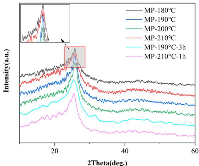
Fig. 10 XRD pattern of sedimentation products of mesophase pitch at the bottom.
