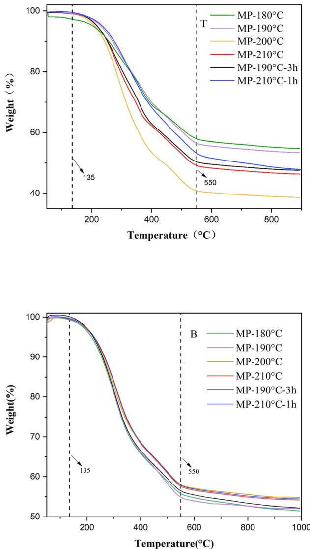
Fig. 7 TG curves of sedimentation products: T, the top of mesophase pitch; B, the bottom of mesophase pitch.
