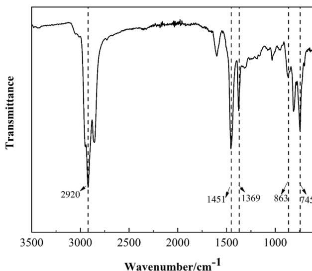
Fig. 1 FTIR spectrum of FCC aromatic-enriched oil.
