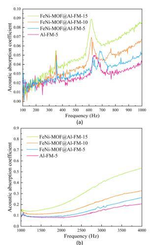
Fig. 7 Acoustic absorption coefficients of FeNi-MOF@Al-FM with different thicknesses: (a) low frequency range; (b) high frequency range.
