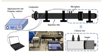
Fig. 1 Schematic diagram and physical image of impedance tube system for testing sound absorption performance of materials.
