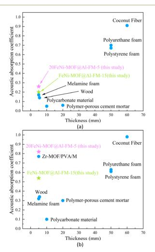
Fig. 10 Sound absorption performance comparative analysis of FeNi-MOF@Al-FM composite vs. conventional materials: (a) sound absorption coefficient at 2000 Hz; (b) sound absorption coefficient at 4000 Hz.
