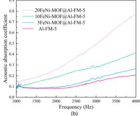
Fig. 8 Acoustic absorption coefficients of FeNi-MOF@Al-FM with different mass ratios: (a) low frequency range; (b) high frequency range.
