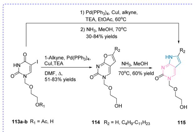
Scheme 24 Synthesis of pyrrolo[2,3-*d*]pyrimidines *via* one-pot coupling.
