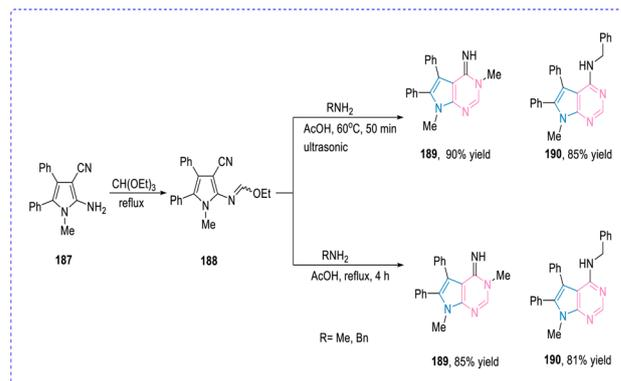
Scheme 36 Synthesis of pyrrolo[2,3-*d*]pyrimidines using catalyst-containing glacial acetic acid or ultrasonic radiation pyrimidine derivatives.Table 9 The antibacterial activity of compounds **189**, **190**
