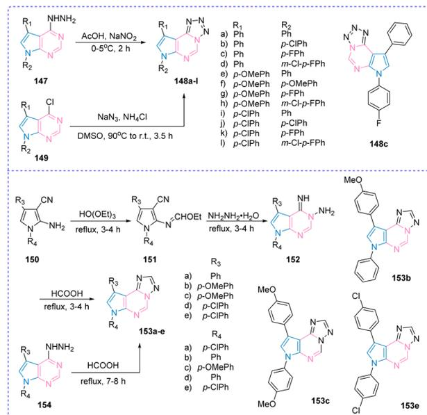
Scheme 29 Synthesis of two cyclized pyrrolo[2,3-*d*]pyrimidines containing triazole and tetrazole.
