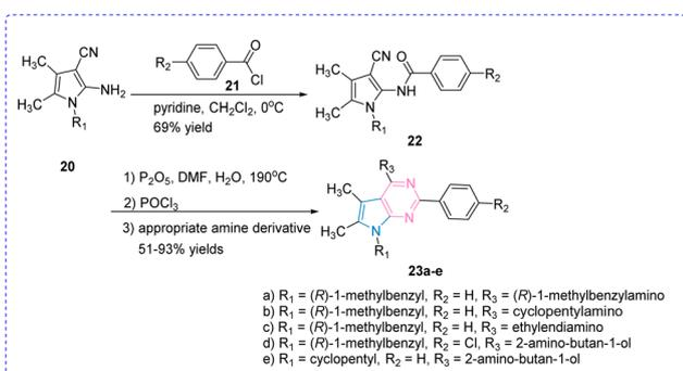
Scheme 5 Synthesis of pyrrolo[2,3-d]pyrimidines using *o*-amino-pyrrorlocarbonitrile.
