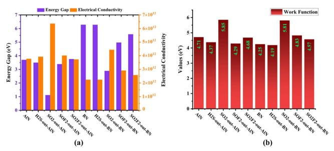
Fig. 10 Comparative study of (a) energy gap and electrical conductivity and (b) work function values of all the systems.
