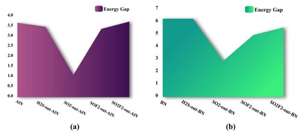
Fig. 2 The variations of energy gap  $(E_q)$  for (a) AlN based systems and (b) BN based systems.
