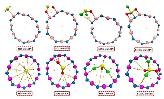
Fig. 8 Visual study of atom in molecules (AIM) analysis showing the important bond critical points (BCPs) between  $SF_6$  decomposed gases and nanorings.
