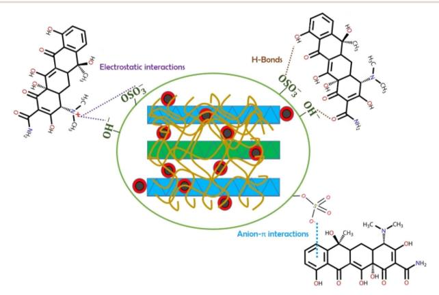
Fig. 11 Interaction mechanism of tetracycline and FACM adsorbent. Reprinted with permission from Amirreza Ahmadpour et al., Inorganic Chemistry Communications, 2023, 156, 111274.© 2023 Elsevier.<sup>108</sup>
