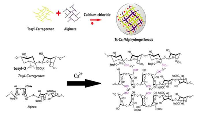
Tosyl-carrageenan system for the removal of heavy metals from wastewater, reprint with permission<sup>90</sup>
