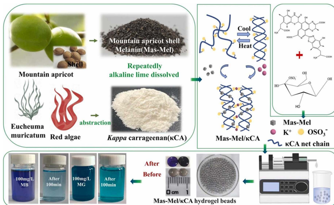
Fig. 10 Synthetic strategy for Mas-Mel/ \kappa -carrageenan hydrogel beads. Reprinted with permission from Rui Hao et al. , Chemical Engineering Research and Design , 2023, 199, 1–10. © 2023 Elsevier. 92
