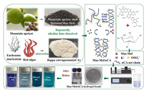
Fig. 10 Synthetic strategy for Mas-Mel/k-carrageenan hydrogel beads. Reprinted with permission from Rui Hao et al., Chemical Engineering Research and Design, 2023, 199, 1–10. © 2023 Elsevier.92
