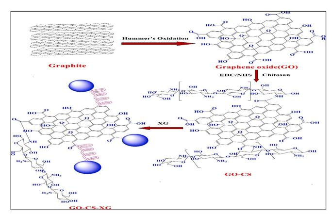
Fig. 13 Schematic illustration of GO-CS-XG synthesis. Reprinted with permission from Kesavan S, et al., International Journal of Biological Macromolecules, 2023, 31, 125322. © 2023 Elsevier.<sup>117</sup>
