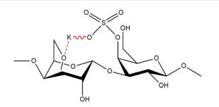
Fig. 7 Intramolecular cation-selective bridging in  $\kappa$ -carrageenan in aqueous solution at low temperatures involves ( $\frac{1}{2}$ ) ionic bonding and (----) electrostatic attractive forces.
