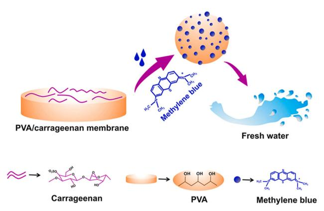
Fig. 9 PVA/carrageenan membranes system for the removal of methylene blue from water. Reprinted with permission from Sabarish Radoor et al., Chemosphere, 2024, **350**, 140990. © 2024 Elsevier.<sup>94</sup>
