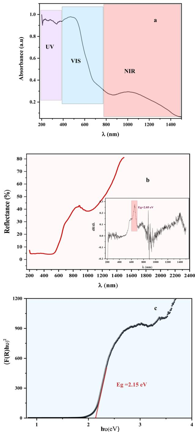
Fig. 4 Absorbance spectra (UV-VIS-NIR) versus  $\lambda$  (a), reflectance spectra versus  $\lambda$  (b). The inset shows the  $dR/d\lambda$  versus  $\lambda$  curve and  $(F(R)h\nu)^2$  versus  $h\nu$  (c) for the  $\text{LiMg}_{0.5}\text{Fe}_2\text{O}_4$  sample.
