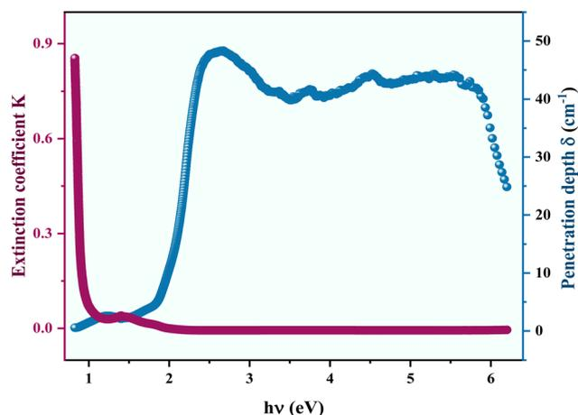
Fig. 6 Evolution of the penetration depth  $\delta$  and the optical extinction  $K$  versus  $h\nu$ .
