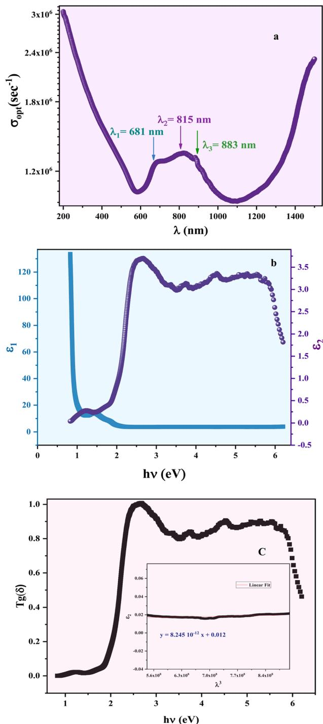
Fig. 8 Optical conductivity  $\sigma_{\text{opt}}$  as a function of  $\lambda$  (a), real and imaginary parts of the dielectric constant of *versus*  $h\nu$ . Represents the energy loss of the light (c). The inset imaginary part of the dielectric constant as a function of  $\lambda^3$  (c).
