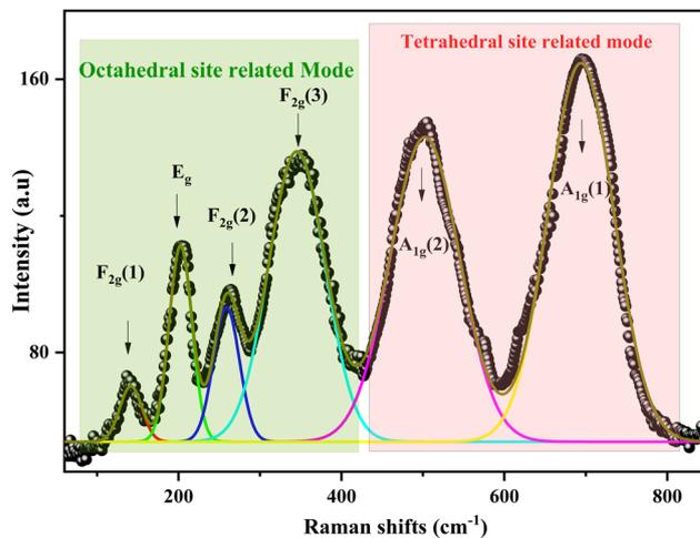
Fig. 2 Raman of  $\text{LiMg}_{0.5}\text{Fe}_2\text{O}_4$ .
