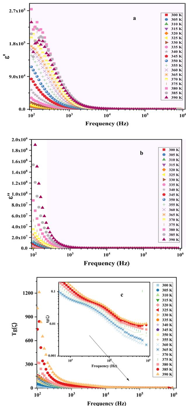
Fig. 11 (a) The dielectric data of the real permittivity ( $\epsilon'$ ), (b) the recorded dielectric data of the imaginary permittivity ( $\epsilon''$ ), (c) loss tangent versus frequencies at several temperatures [300–390 K] for the synthesized ferrite.
