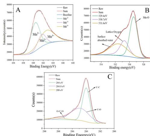
Fig. 2 High resolution XPS spectra of Mn<sub>2</sub>p<sub>3/2</sub> (A), O1s (B) and C1s (C).
