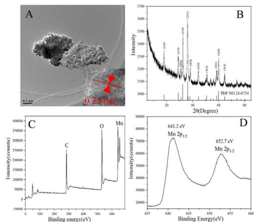
Fig. 1 TEM images (A), XRD (B), XPS survey (C) of MBC, high resolution XPS (D) of Mn 2p.
