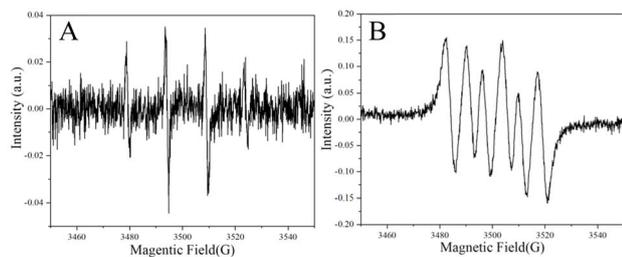
Fig. 8 Situ EPR spectra for detection of  $\cdot\text{OH}$  (A) and  $\cdot\text{O}_2^-$  (B) radicals under light illumination.
