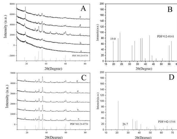
Fig. 3 The effect of the mass ratios of biochar to MnSO<sub>4</sub> (A), stirring time (C) on the XRD of MBC, and the standard XRD of MnO<sub>2</sub> (B and D). (The mass ratios of biochar to MnSO<sub>4</sub> are 1 : 2, 2 : 5, 1 : 3, 2 : 7, and 1 : 4. The stirring times are 0.5, 1, 2, 3, 4 h).
