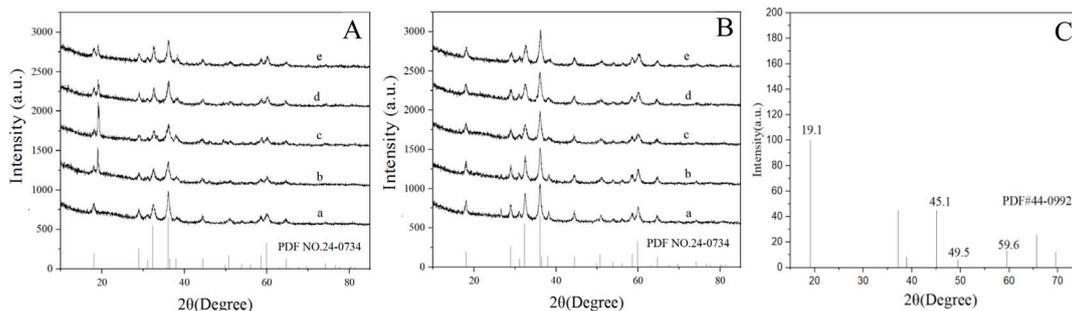
Fig. 4 The effect of the dropping speeds (A) and dosages (B) of  $\text{NH}_3 \text{H}_2\text{O}$  added on the XRD of MBC, the standard XRD of  $\text{MnO}_2$  (C). (The dropping speeds are 5, 10, 15, 20 and 25 drip per minute. The dosages are 1.34, 2.00, 2.67, 3.34 and 4.01 mol  $\text{L}^{-1}$ ).
