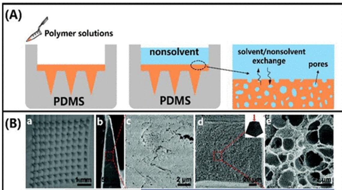
Fig. 5 Process and pictures of PPMNs prepared by the nonsolvent induced phase separation method. (A): The process of preparing PPMNs by nonsolvent induced phase separation. (B): Structural characterization of porous microneedles made of CA (a–e): optical microscopy images of the microneedle arrays (a) and surface (b–c) and cross-sectional (d and e) SEM images of microneedles at different magnifications. Reproduced with permission from<sup>11</sup> [Copyright© 2023, ACS].
