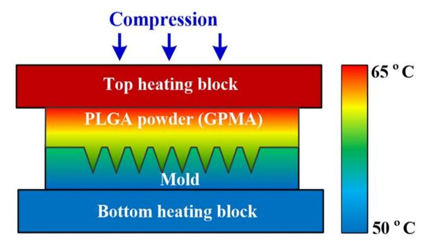
Fig. 6 Schematic illustration of modified hot embossing process setup for the GMPA fabrication. Reproduced with permission from 6 [Copyright ©2019, Elsevier].
