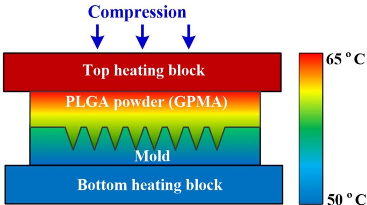
Fig. 6 Schematic illustration of modified hot embossing process setup for the GMPA fabrication. Reproduced with permission from<sup>16</sup> [Copyright ©2019, Elsevier].
