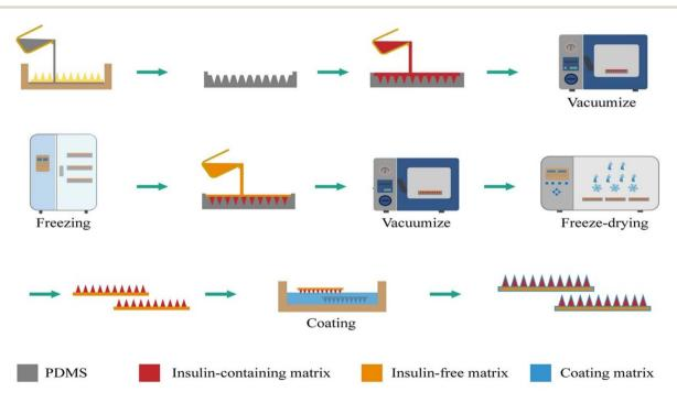
Fig. 7 Schematic illustration of freeze-drying method for fabrication of microneedle loaded with insulin. Reproduced with permission from <sup>49</sup> [Copyright ©2024, Springer Nature].
