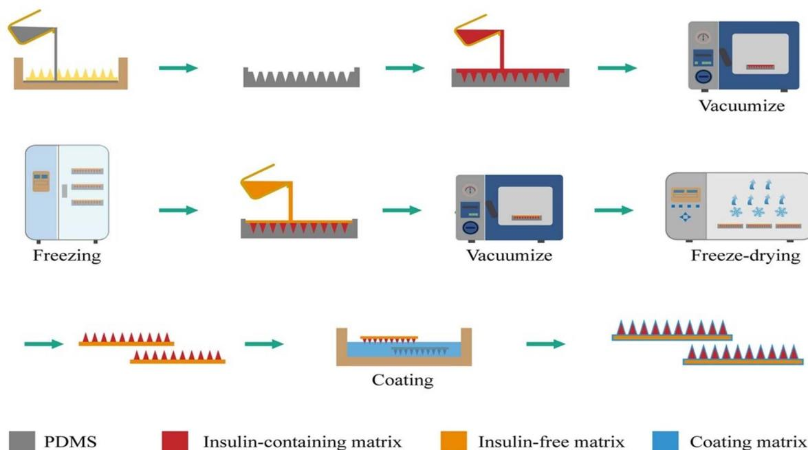
Fig. 7 Schematic illustration of freeze-drying method for fabrication of microneedle loaded with insulin. Reproduced with permission from<sup>49</sup> [Copyright ©2024, Springer Nature].
