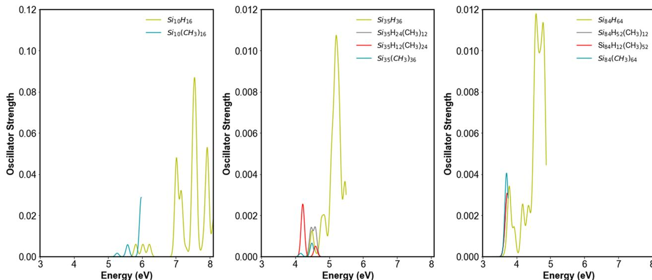
Fig. 10 Absorption spectra of the hydrogen-terminated SiNPs versus their partially methyl-terminated and fully methyl-terminated counterparts as predicted using TD-DFT,  $C_1$  symmetry, the B3LYP functional, def2-SVP basis set and a Gaussian broadening of 0.05 eV.
