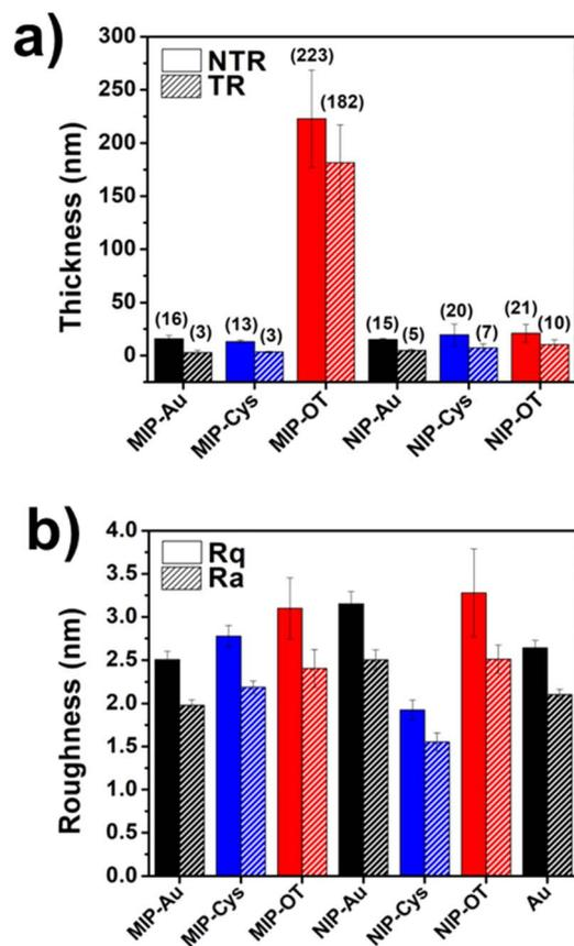
Fig. 3 (a) Thickness values of the polymer coatings. The abbreviations NTR and TR stand for no template removal and template removal steps. (b) Roughness values expressed as  $R_q$  (RMS roughness) and  $R_a$  (average roughness) of the polymer coatings after template removal step obtained from  $1 \times 1 \mu\text{m}^2$  AFM images.
