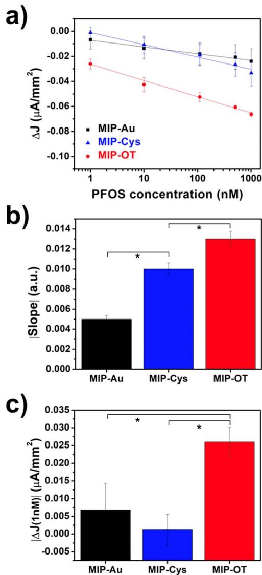
Fig. 5 (a) Calibration curves of MIP samples. Straight lines are the linear fittings. (b) Absolute slope values of the linear fittings. (c) Absolute  $\Delta J$  values at 1 nM PFOS. Statistical analysis was performed using on-way ANOVA; differences were considered significant when  $P \leq 0.05$  (\*\*).
