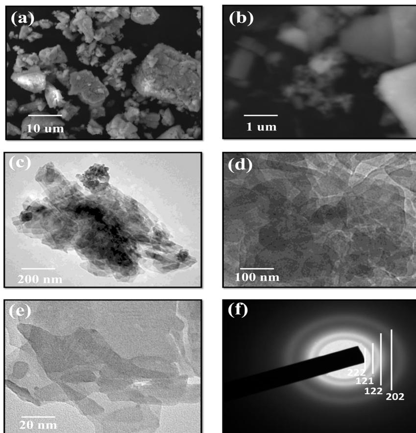
Fig. 3 (a and b) Low and high resolution FESEM images, (c and d) TEM images at 200 nm and 100 nm, (e and f) HRTEM image and SAED pattern of Eu-Ag<sub>2</sub>Se nanoparticles.
