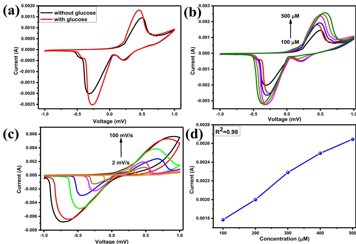
**Fig. 6** (a) CV of the Eu–Ag<sub>2</sub>Se nanoparticles without and with glucose concentration performed in the presence of 0.1 M of NaOH electrolytic solution, (b) CV of the Eu–Ag<sub>2</sub>Se nanoparticles at different concentration of glucose molecules, (c) CV of the Eu–Ag<sub>2</sub>Se nanoparticles at different scan rates and (d) graph between oxidation peak current with their correspondence glucose concentration.
