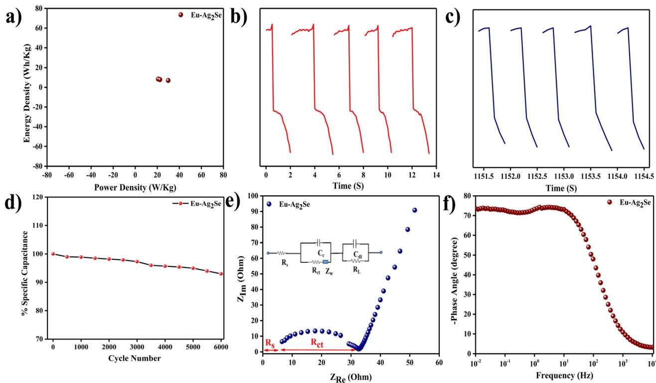
Fig. 5 (a) Plot between energy density with power density, (b) charge and discharge time of Eu-Ag<sub>2</sub>Se of first five cycles, (c) charge and discharge time of Eu-Ag<sub>2</sub>Se of last five cycles, (d) plot between specific capacitances with various cycle numbers, (e) Nyquist plot of Eu-Ag<sub>2</sub>Se, (f) Bode plot of Eu-Ag<sub>2</sub>Se at frequency range 0.01 Hz to 10 kHz.
