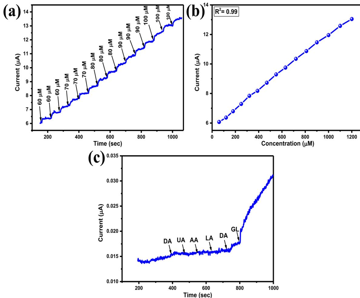
Fig. 7 (a) IT curve of Eu-Ag<sub>2</sub>Se nanoparticles (b) calibration curve of Eu-Ag<sub>2</sub>Se nanoparticles. (c) Interference study of Eu-Ag<sub>2</sub>Se nanoparticles.
