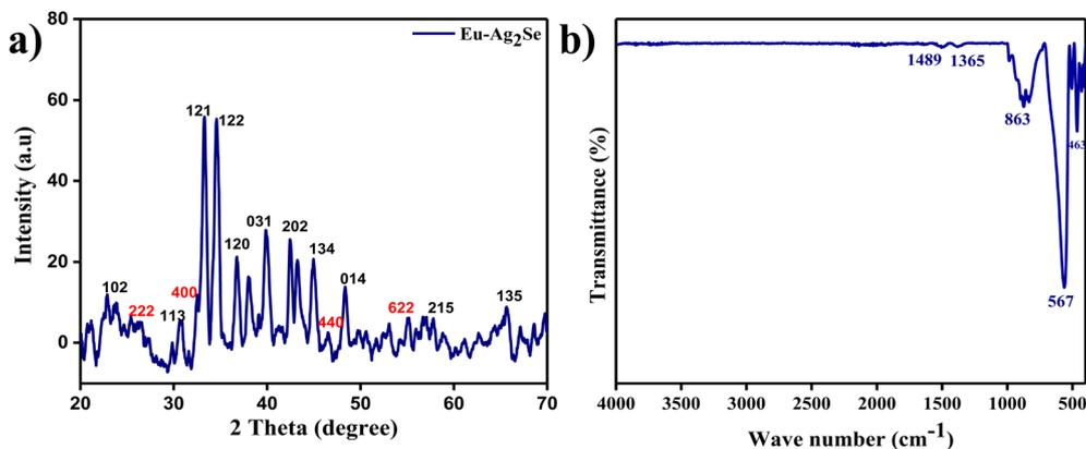
Fig. 2 (a) XRD pattern of Eu- $\text{Ag}_2\text{Se}$  nanoparticles (b) FTIR spectrum of Eu- $\text{Ag}_2\text{Se}$  nanoparticles.
