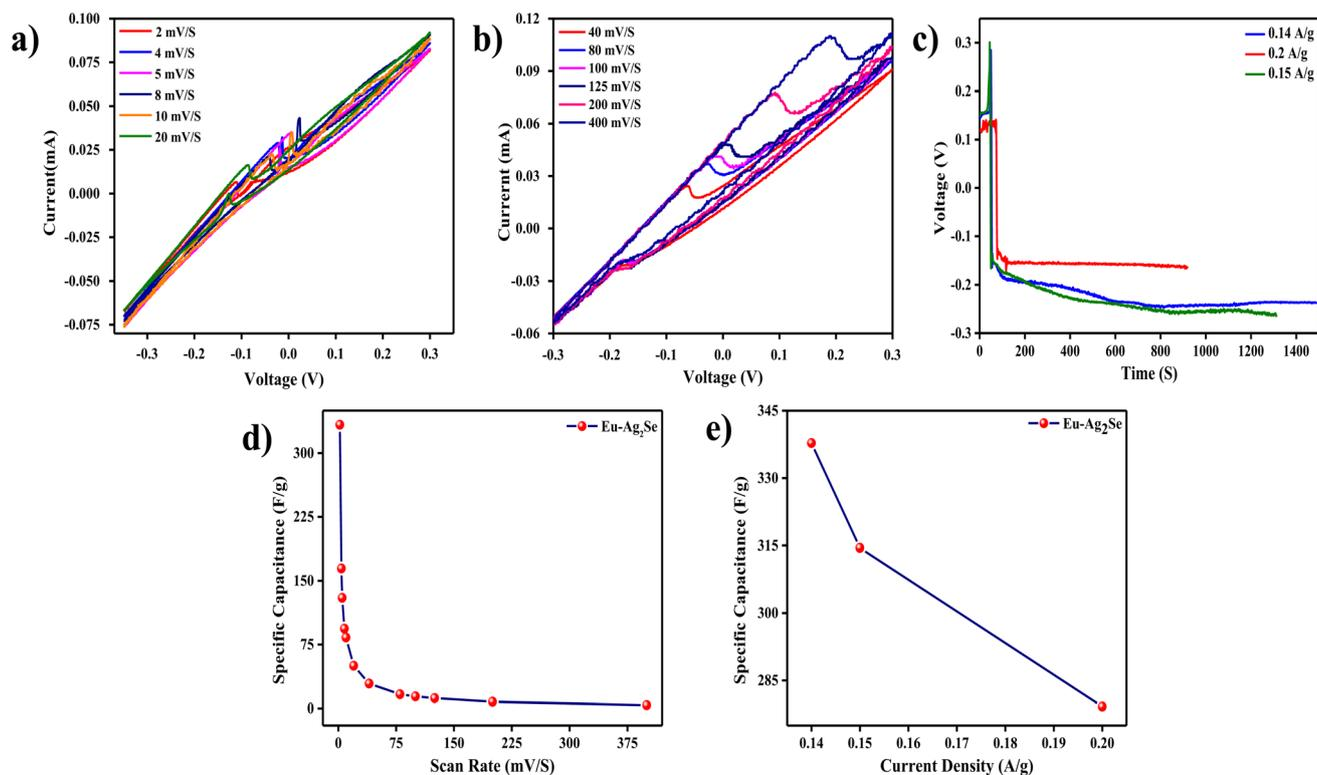
Fig. 4 (a and b) CV curves of Eu-Ag<sub>2</sub>Se nanoparticles at different scan rates (2–400) mV S<sup>-1</sup>, (c) GCD curves of Eu-Ag<sub>2</sub>Se nanoparticles at different current densities (d) plot between specific capacitances with various scan rates (e) plot between specific capacitances with various current densities.
