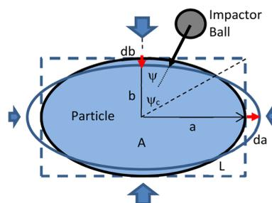
Fig. 8 Schematic arrangement for plastic deformation (not to scale). (a and b) Half-axes of ellipsoidal particle  $da, db$ : elongation and compression deformation of half axes  $\psi, \psi_c$ : incidence angle and critical incidence angle  $A$ : particle area.
