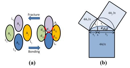
Fig. 6 (a) Particle bonding and fracture. (b) Fracture size relationship and probability distribution.
