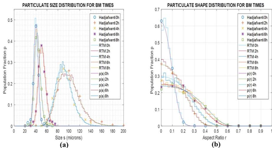
Fig. 11 Population fraction pdfs  $p$  for BM tests using Hadjiaf Kenti *et al.*<sup>11</sup> (Al–Ni 1 : 3, 300 rpm) (a) literature data, RTM simulations and stochastic results of size  $s$  for various times  $t$  (b) literature data, RTM simulations and stochastic results of aspect ratio  $r$  for various times  $t$ .
