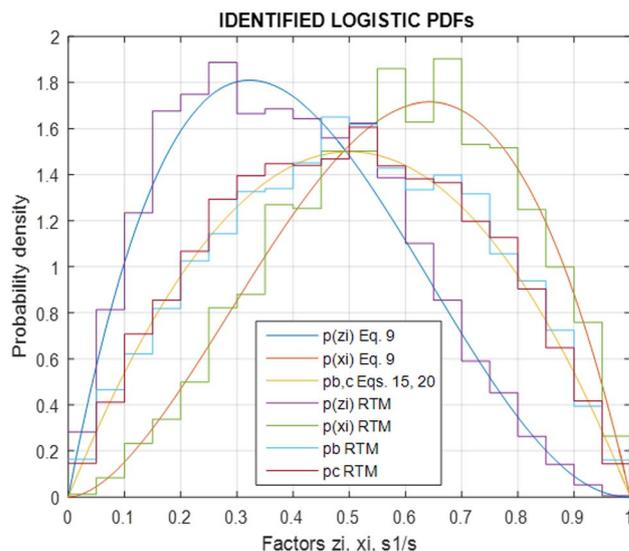
Fig. 7 Probability density functions of tribological factor  $\zeta$ , plasticity factor  $\xi$  and fracture size  $s_1/s$  resulting from real-time model and fitted by eqn (9), (15) and (20).
