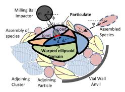
Fig. 4 Particulate with assembly of adjoining particles, impactor and anvil (not to scale).
