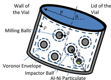
Fig. 5 Collision schematic arrangement (not to scale).
