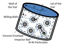
Fig. 5 Collison schematic arrangement (not to scale).
