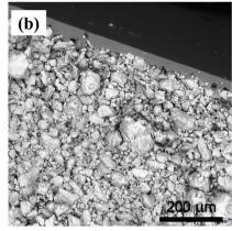
Fig. 1 SEM micrographs of Al-Ni (1:1) composite particulates by BM (300 rpm): (a) loose particulate external and internal structure (after 13 hours of BM)<sup>10</sup> (b) compacted into 800 μm-thick foils sandwiched with Al overlayers (9 hours of BM).<sup>12</sup>
