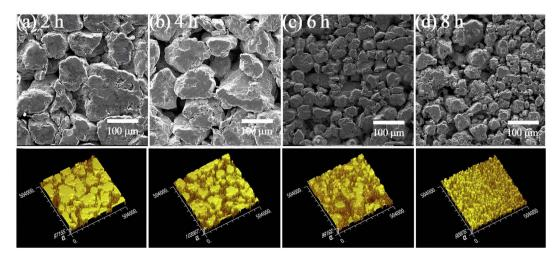
Fig. 2 Micrographs of Al–Ni (1:3) particles after (a) 2 h, (b) 4 h, (c) 6 h and (d) 8 h of BM at 300 rpm<sup>11</sup> (Top row): SEM secondary electron (SE) images; (Bottom row): Laser profilometer scans.
