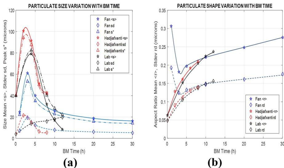
Fig. 12 Time variation of particle size and shape in Fan,<sup>13</sup> Hadjiaf Kenti<sup>11</sup> and lab BM tests (a) mean  $s$ , standard deviation  $s_d$  and most probable value  $s^*$  of size  $s$  (b) mean  $r$  and standard deviation  $r_d$  of aspect ratio  $r$ .
