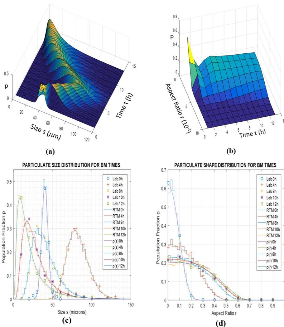
Fig. 9 Population fraction pdfs  $p$  for calibration BM tests (Al-Ni 1:1, 300 rpm) (a) stochastic model results for  $p$  as function of size  $s$  and time  $t$  b. Stochastic model results for  $p$  as function of aspect ratio  $r$  and time  $t$  (c) laboratory data, RTM simulations and stochastic results of size  $s$  for various times  $t$  (d) laboratory data, RTM simulations and stochastic results of aspect ratio  $r$  for various times  $t$ .
