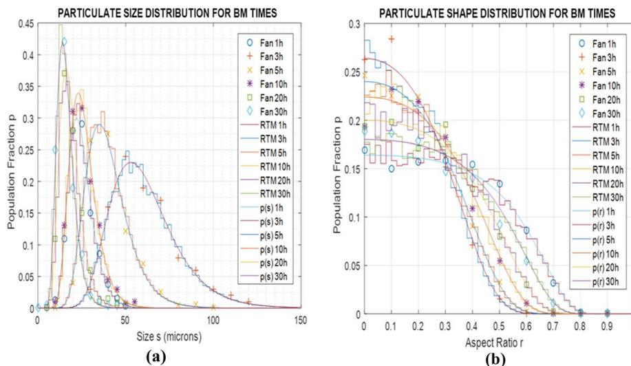
Fig. 10 Population fraction pdfs  $p$  for validation BM tests using Fan *et al.*<sup>13</sup> (Al–Ni 1 : 1, 400 rpm) (a) literature data, RTM simulations and stochastic results of size  $s$  for various times  $t$  (b) literature data, RTM simulations and stochastic results of aspect ratio  $r$  for various times  $t$ .
