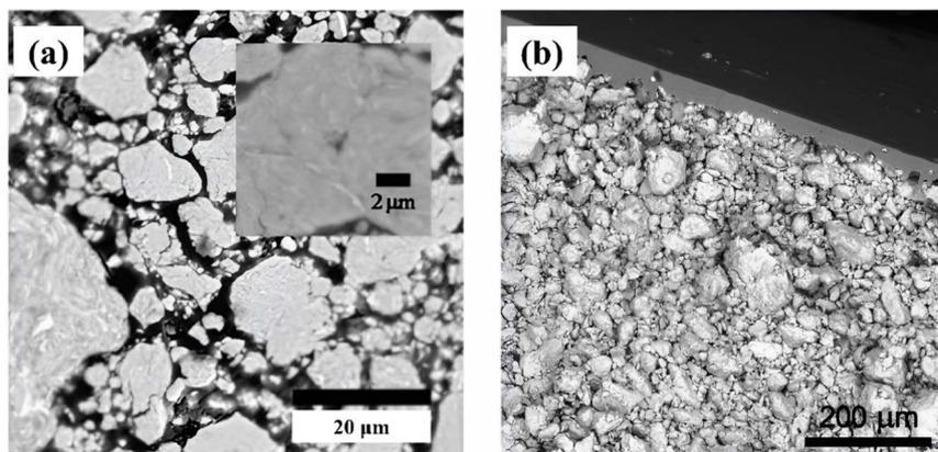
Fig. 1 SEM micrographs of Al–Ni (1 : 1) composite particulates by BM (300 rpm): (a) loose particulate external and internal structure (after 13 hours of BM)<sup>10</sup> (b) compacted into 800  $\mu\text{m}$ -thick foils sandwiched with Al overlayers (9 hours of BM).<sup>12</sup>
