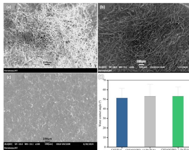
Fig. 3 SEM images of (a) CNF, (b) CNF/PVA, (c) and CNF/rGO/WO<sub>3</sub> membrane, and (d) water contact angles of the CNF/PVA, CNF/rGO/WO<sub>3</sub> (0.5% PVA), and the CNF/rGO/WO<sub>3</sub> (2% PVA) membrane.
