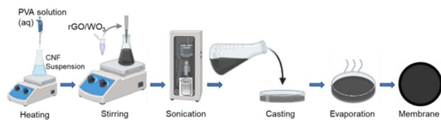
Fig. 2 Schematic representation of membrane fabrication by solution casting.
