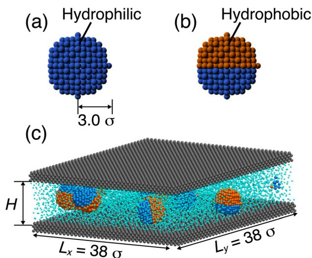
Fig. 1 Simulation models of (a) HI NP and (b) Janus NP with radius  $R = 3.0 \sigma$ . (c) Representative snapshot of a nanofluid confined between two solid walls with channel height  $H$ . In all panels, hydrophilic beads are shown in blue, hydrophobic beads in orange, solvent beads in cyan, and wall beads in gray.
