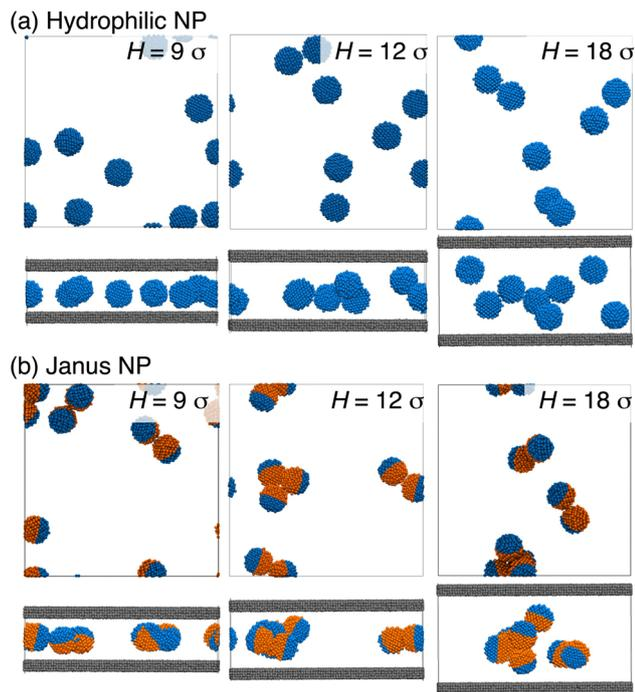
Fig. 2 Representative snapshots of (a) homogeneous HI NPs and (b) Janus NPs at various channel heights,  $H$ , as indicated. In each panel, the top image shows the side view, while the bottom image presents the view along the direction normal to the wall surface.
