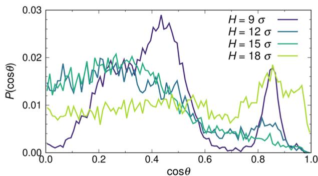
Fig. 3 Orientational distributions,  $P(\cos\theta)$ , of confined Janus NPs at various channel heights,  $H$ , as indicated.  $\theta$  is defined as the angle between the surface normal of the wall (along the  $z$ -direction) and the unit vector from the hydrophilic to the hydrophobic pole.
