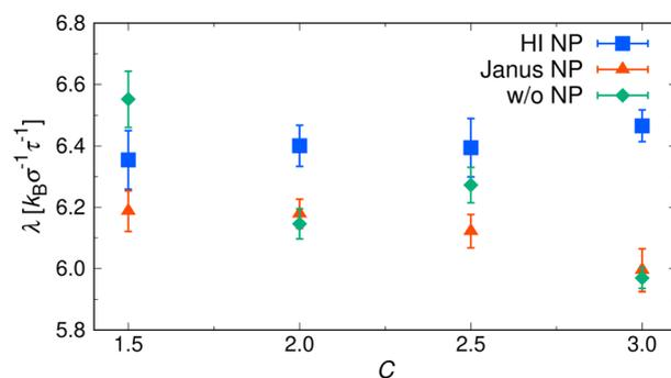
Fig. 4 Thermal conductivity,  $\lambda$  of nanofluids as functions of the confinement ratio  $C$ . Blue squares: hydrophilic NPs, orange triangles: Janus NPs, green diamonds: pure solvent (without NPs).
