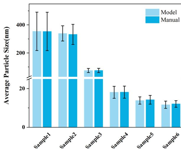
**Fig. 6** Comparison between model and manual particle size measurements.
