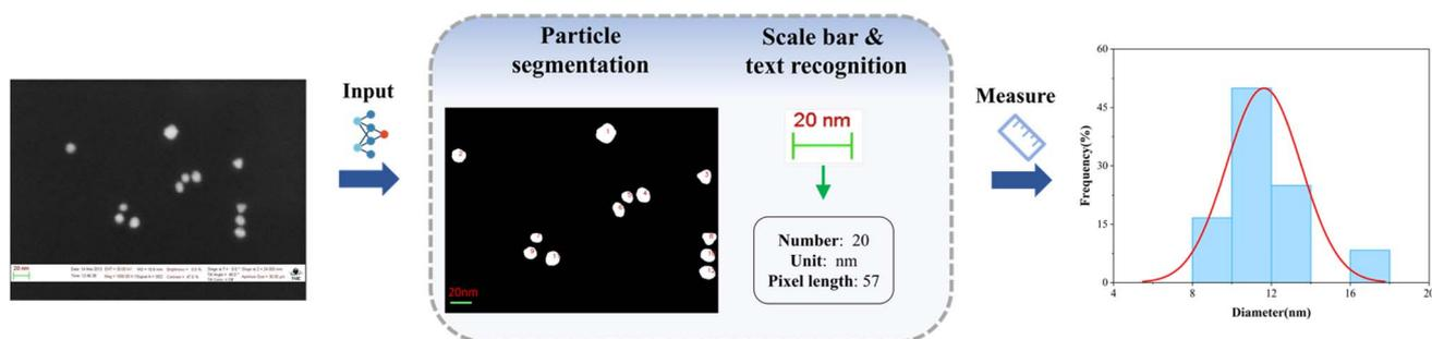
Fig. 3 Overall flowchart of nanoparticle size measurement.
