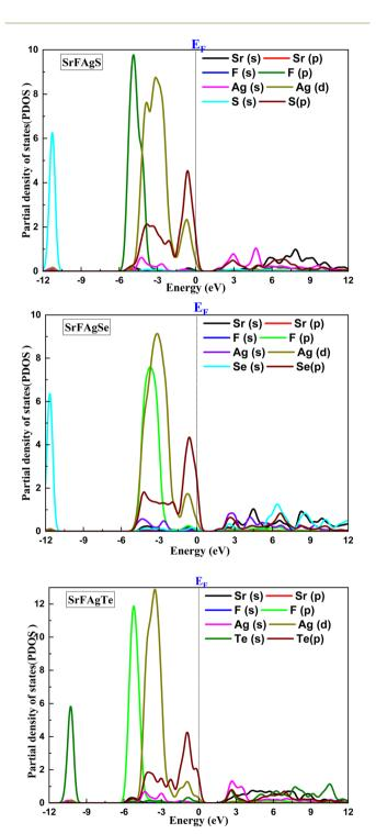
Fig. 4 Partial density of states (PDOS) for SrFAgX compounds, illustrating strong Ag-d and X-p orbital hybridization near the Fermi level, which contributes to the observed electronic properties.
