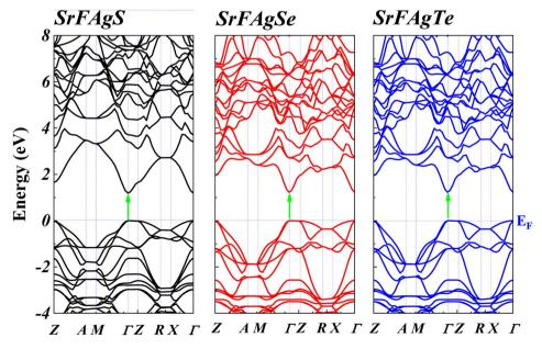
Fig. 2 Electronic band structures of SrFAgX (X = S, Se, Te) along high-symmetry directions, indicating direct band gaps that decrease from S to Te due to enhanced orbital overlap and chalcogen substitution effects.
