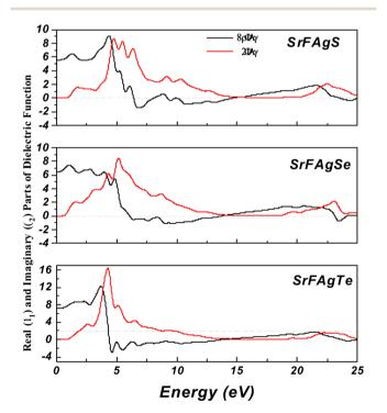
Fig. 5 Real ( $\varepsilon_1$ ) and imaginary ( $\varepsilon_2$ ) parts of the complex dielectric function for SrFAgS, SrFAgSe, and SrFAgTe as functions of photon energy, highlighting enhanced optical response and static dielectric constant in SrFAgTe compared to its lighter counterparts.
