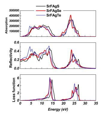
**Fig. 6** Absorption spectra, reflectivity, and energy loss function of SrFAgX compounds, showing stronger absorption in the visible-UV range and higher energy loss peaks in SrFAgTe, indicating stronger plasmonic activity.
