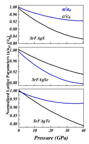
Fig. 1 Pressure dependent normalized lattice parameters ( $a/a_0$  and  $c/c_0$ ) for SrFAgSe, SrFAgSe, and SrFAgTe compounds, showing anisotropic compressibility with greater contraction along the c-axis than the a-axis under increasing pressure.
