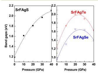
Fig. 3 Evolution of electronic band gaps of SrFAgX compounds under applied pressure up to 40 GPa, revealing a monotonic increase for SrFAqS and non-monotonic behavior for SrFAqSe and SrFAqTe.
