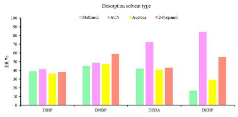
Fig. 4 Selection of desorption solvent type. Extraction conditions: are the same as those used in Fig. S4, except 20% (w/v)  $Na_2SO_4$  was used as the salting-out agent in the  $D\mu SPE$  step.
