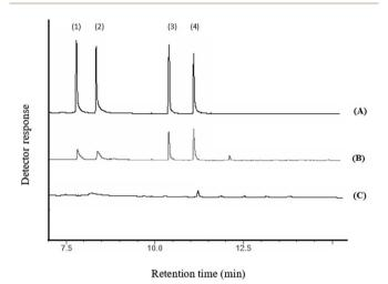
Fig. 6 GC-FID chromatograms of standard solution of the analytes 500 mg  $L^{-1}$  of each in methanol (A), agueous solution (500 µg of each) (B), and wound disinfectant (C). The proposed method was applied on them and 1 µL of the final sedimented organic phase was injected into GC-FID, except chromatogram (A) in which organic phase was injected directly. Peaks identification: (1) DIBP, (2) DNBP, (3) DEHA, and (4) DEHP.
