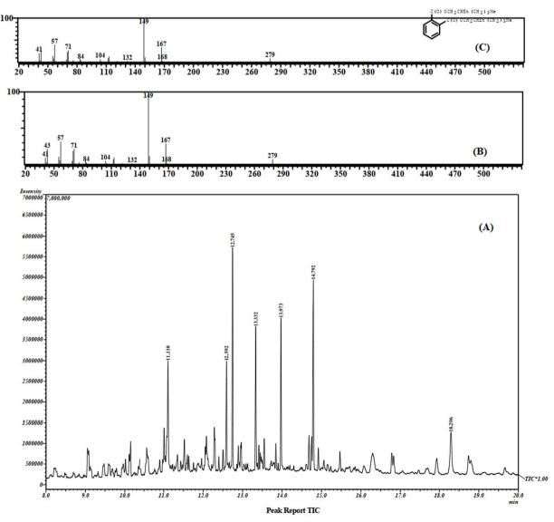
Fig. 7 Typical GC-MS chromatogram of disinfectant after performing the proposed method (A), mass spectrum of DEHP (B), and scan 3594 (retention time 13.98 min) (C).
