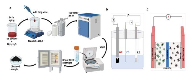
Scheme 1 (a) An illustration of the synthesis procedure for the preparation of powder samples *via* a hydrothermal method, (b) an illustration of the 3-electrode setup and (c) the construction of the symmetric supercapacitor device.
