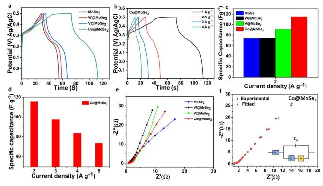
Fig. 6 (a) GCD plots for all samples at  $1 \text{ A g}^{-1}$ , (b) GCD plots of Co@MoSe<sub>2</sub> at varied current densities (A  $g^{-1}$ ), (c and d) current density vs. specific capacitance plots, (e) Nyquist plots corresponding to all prepared samples, and (f) experimental and fitted data for Co@MoSe2 (the inset displays the equivalent fitted circuit).
