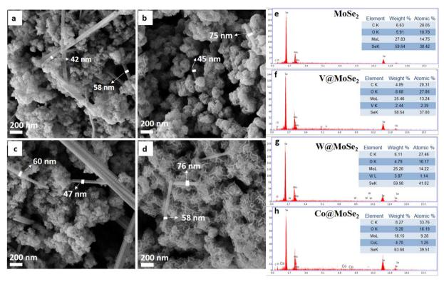
Fig. 2 FESEM images of (a)  $MoSe_2$ , (b)  $V@MoSe_2$ , (c)  $W@MoSe_2$ , and (d)  $Co@MoSe_2$ , and (e-h) EDX spectra confirming the elemental compositions of the samples.
