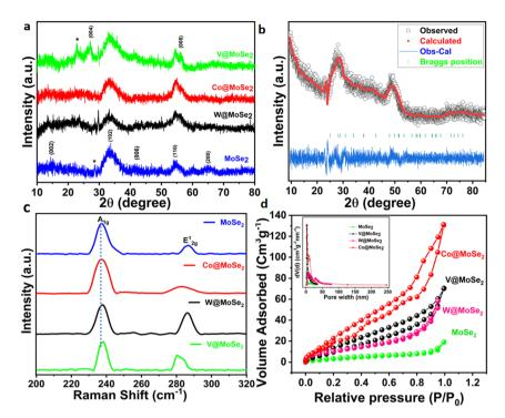
Fig. 1 (a) Powder X-ray diffraction (PXRD) patterns of a pure MoSe<sub>2</sub> sample, W@MoSe<sub>2</sub>, Co@MoSe<sub>2</sub> and V@MoSe<sub>2</sub>. (b) Rietveld refinement performed on the XRD data of a pure MoSe<sub>2</sub> sample. (c) Raman spectra of MoSe<sub>2</sub>, W@MoSe<sub>2</sub>, Co@MoSe<sub>2</sub>, and V@MoSe<sub>2</sub>. (d) BET results and the corresponding BJH plots (inset).
