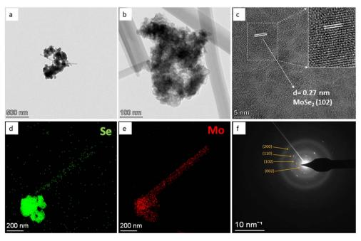
Fig. 3 (a-c) HRTEM images of a pure sample, (d and e) element mapping of Mo and Se, and (f) the SAED pattern of MoSe<sub>2</sub>.
