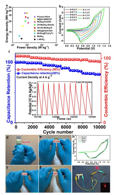
Fig. 8 (a) Ragone plot of the device compared with the reported literature, (b) CV curves observed over different potential windows, (c) cycling stability and coulombic efficiency of the  $Co@MoSe_2$  SSD at a current density of 4 A  $g^{-1}$  (the inset shows the GCD curves from the last ten cycles), (d-g) pictorial illustrations of the bending and twisting of the SSD and (h) related CV curves, and (i) photographic evidence of a red LED being lit by SSDs in series.
