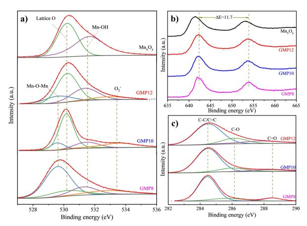
Fig. 3 XPS spectra of  $Mn_xO_v$  and GMP8-GMP12 nanocomposite samples: (a) O 1s; (b) Mn 2p and (c) C 1s.
