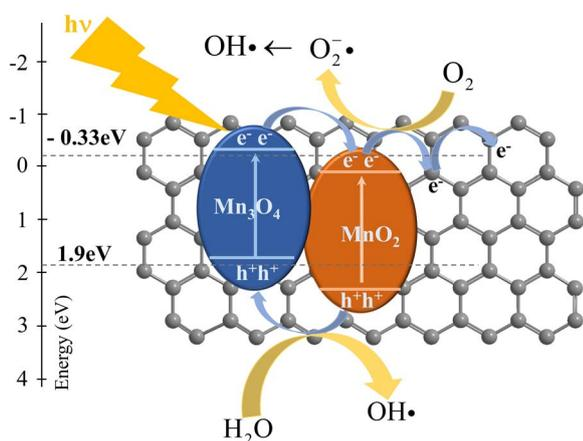
Fig. 7 Mechanism of MB photocatalysis by GMP10.
