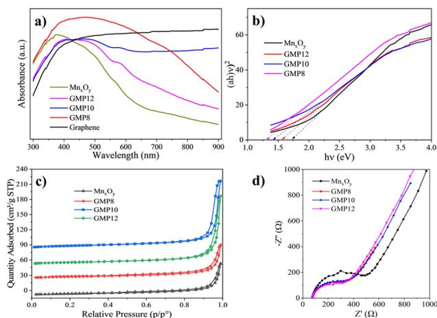
Fig. 5 (a) Diffuse reflectance absorption spectrum; (b) Tauc plots; (c)  $\text{N}_2$  adsorption–desorption isotherms and (d) Nyquist plot of graphene,  $\text{Mn}_x\text{O}_y$ , and GMP8–GMP12 composite samples.
