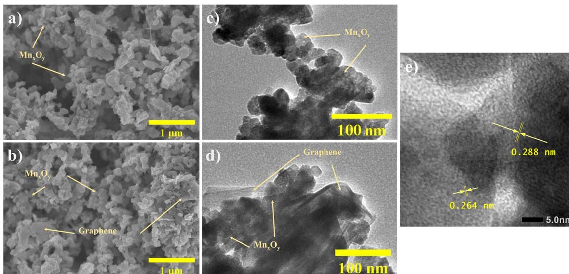
Fig. 4 SEM (a and b) and TEM (c and d) images of manganese oxide and the GMP10 composite material; and (e) HR-TEM images of the GMP10 composite material.
