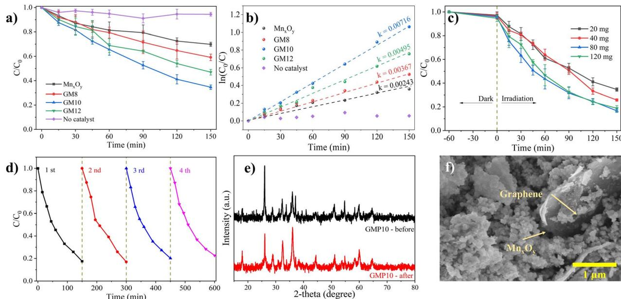
Fig. 6 Comparison of photocatalytic ability of  $Mn_xO_y$  and GMP8–GMP12 composite catalysts (catalyst dosage:  $m = 20$  mg) for degrading MB dye: (a)  $C/C_0$  plot and (b)  $\ln(C_0/C)$  plot; (c) effects of the amount of GMP10 for MB decomposition; (d) photocatalytic cycling experiments of GMP10, using 80 mg of catalyst; (e) XRD patterns of GMP10 before and after stability test and (f) SEM of GMP10 after stability test.
