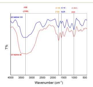
Fig. 2 FTIR spectra of the synthesized GT-NZVAI 40 and GT-NZVAI 100.
