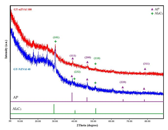
Fig. 3 XRD patterns of the synthesized GT-NZVAI (40 and 100).
