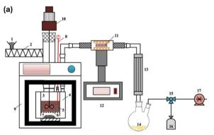
(1) hopper; (2) auger; (3) inner vessel; (4) outer vessel; (5) ball-type SiC; (6) sieve bottom; (7) char; (8) thermocouple; (9) microwave oven; (10) electrical agitator; (11) catalytic bed; (12) tubular microwave heater; (13) condenser; (14) oil-collecting flask; (15) three-way valve; (16) gas sampling bag; (17) vacuum pump
