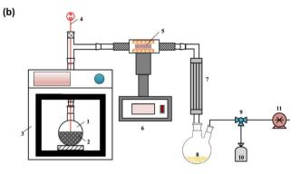
(1) quartz flask; (2) feedstock mixed with SiC; (3) microwave oven; (4) thermocouple; (5) catalytic bed; (6) tubular microwave heater; (7) condenser; (8) oil-collecting flask; (9) three-way valve; (10) gas sampling bag; (11) vacuum pump
