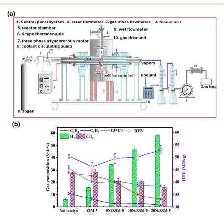
Fig. 5 (a) Schematic overview of the semi-batch rotary reactor and (b) gas composition, specifically H<sub>2</sub>. Reproduced with permission from ref. 116. Copyright 2024, Elsevier.
