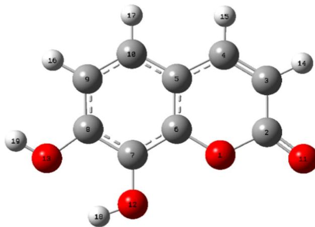
Fig. 3 Daphnetin (DAPH) optimized structure by DFT B3LYP/6-311++G (d, p), using methanol as solvent,  $E = -647.38$  au ( $-406237.42$  kcal mol<sup>-1</sup>).
