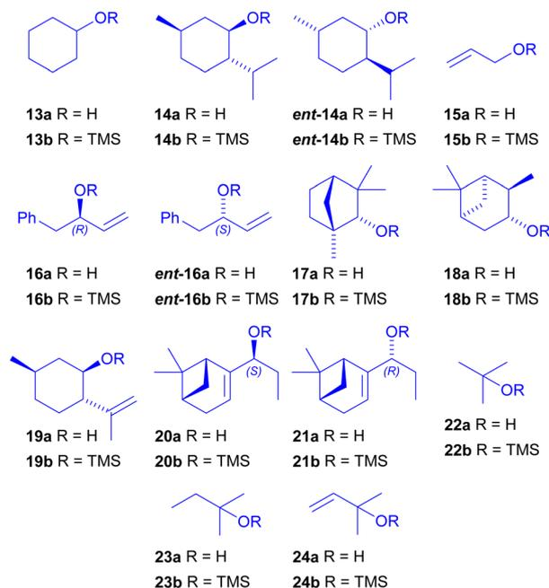
Scheme 5 Alcohols and TMS ethers used in multicomponent Hosomi–Sakurai reactions of Tables 3 and 4.
