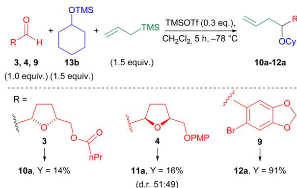
Scheme 3 Preliminary results. TMSOTf (trimethylsilyl trifluoromethanesulfonate) was used as freshly prepared 0.3 M solution in  $\text{CH}_2\text{Cl}_2$ ; equiv. = equivalent; Cy = cyclohexyl; Y = yield; d.r. = diastereomeric ratio.
