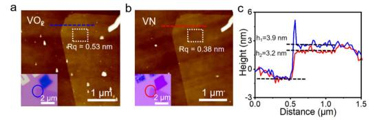
Fig. 2 AFM characterization of a sample film before  $(VO_2)$  and after nitride (VN). (a) and (b) Are AFM images at the same place on  $VO_2$  and VN sample (location marked by circle region in the left inset optical microscopy). (c) AFM height profile (along blue and red dashed lines in (a) and (b)) suggests the thickness reduced after nitriding.
