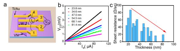
Fig. 5 Impact of thickness to the electrical properties of VN film. (a) A schematic illustration of fabricating a four-electrode configuration on a VN film on  $SiO_2/Si$  substrate. (b) Room-temperature I-V curves of the samples with different thickness. (c) Plot of  $R_s$  versus thickness for VN.
