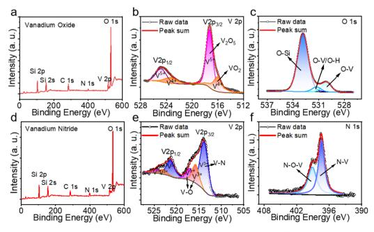
Fig. 4 X-ray photoelectron spectroscope (XPS) spectra of the prepared VO<sub>2</sub> and VN samples on SiO<sub>2</sub>/Si substrates showing survey spectrums in (a) and (d). High-resolution, de-convoluted XPS spectra of (b) V 2p and (c) O 1s peaks for vanadium oxide, (e) V 2p and N 1s (f) for vanadium nitride.
