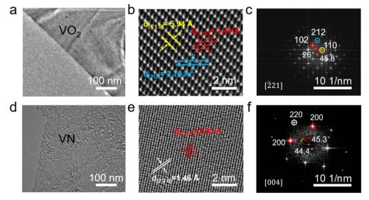
Fig. 3 TEM characterizations of  $VO_2$  and VN film. (a) Low-magnification TEM image of  $VO_2$  film transferred to a TEM grid. (b) HRTEM images of  $VO_2$  film. (c) The corresponding FFT patterns to (b), shows zone axis [ $\bar{2}21$ ]. (d) Low-magnification TEM image of VN film transferred to a TEM grid. (e) HRTEM images of VN film. (f) The corresponding FFT patterns to (e), shows the cubic structure of vanadium nitride belonging to the zone axis [ $\bar{0}04$ ].
