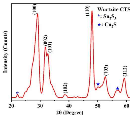
Fig. 1 The XRD pattern of deposited CTS TF.
