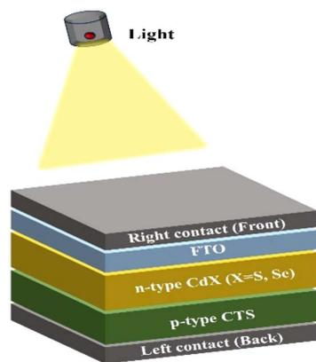
Fig. 6 Schematic diagram of proposed device structure.
