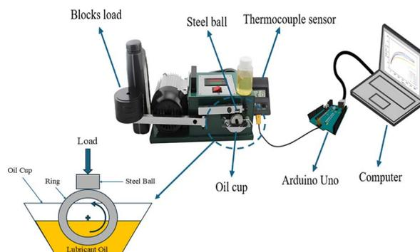
Fig. 3 Experimental set up for abrasion tester.
