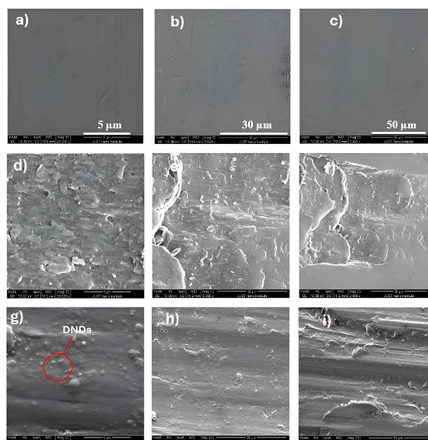
Fig. 9 The SEM images of the standard steel balls were characterized before and after abrasion testing: (a–c) standard steel balls before abrasion testing at 5, 30 and 50  $\mu\text{m}$ , (d–f) standard steel balls after abrasion testing using pure oil at 5, 30 and 50  $\mu\text{m}$  and (g–i) standard steel balls after abrasion testing using nano-lubricant oil 0.005 wt% at 5, 30 and 50  $\mu\text{m}$ .
