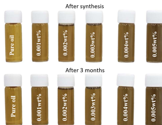
Fig. 13 High stability for nano-lubricants appears after synthesis and after 3 months of synthesis.
