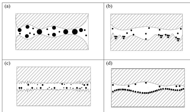
Fig. 1 Lubricating mechanisms by NPs based lubricant: (a) rolling effect. (b) Mending effect. (c) Polishing effect. (d) Protective film.
