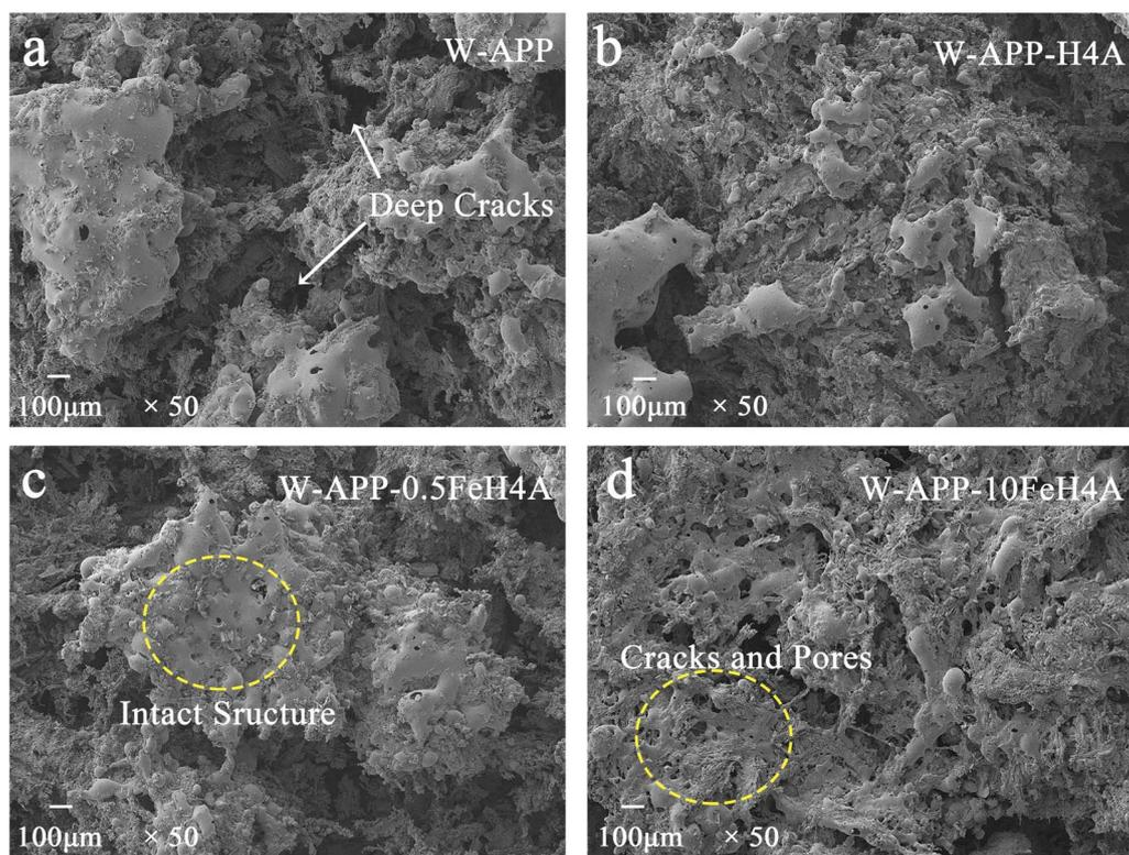
Fig. 9 Char residue of different samples after CCT ((a) W-APP; (b) W-APP-H4A; (c) W-APP-0.5FeH4A; (d) W-APP-10FeH4A).
