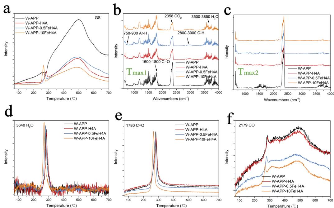
Fig. 8 (a) Gram-Schmidt (GS) curves and FTIR spectra at (b)  $T_{\max 1}$  and (c)  $T_{\max 2}$  of different samples. (d) Water at  $3640\text{ cm}^{-1}$ , (e) C=O compounds at  $1780\text{ cm}^{-1}$ , and (f) CO at  $2179\text{ cm}^{-1}$  evolved during the thermal decomposition process.
