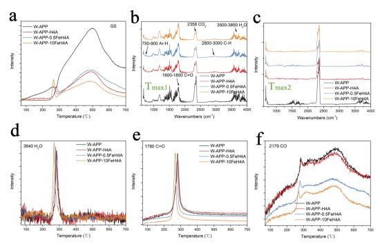
Fig. 8 (a) Gram-Schmidt (GS) curves and FTIR spectra at (b)  $T_{\text{max1}}$  and (c)  $T_{\text{max2}}$  of different samples. (d) Water at 3640 cm<sup>-1</sup>, (e) C=O compounds at 1780 cm<sup>-1</sup>, and (f) CO at 2179 cm<sup>-1</sup> evolved during the thermal decomposition process.
