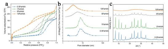
Fig. 2 (a) N<sub>2</sub> adsorption-desorption isotherms, (b) BJH pore diameter distributions, and (c) XRD patterns of H4A zeolites.
