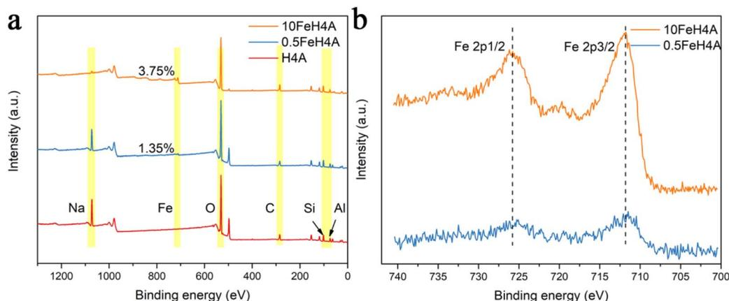
Fig. 3 (a) XPS survey scans and (b) high resolution Fe 2p XPS spectra of samples.
