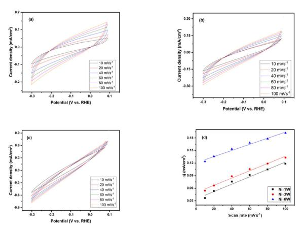
Fig. 9 Cyclic voltammetry curves in 1 mol  $L^{-1}$  KOH at scan rates varying from 10 to 100 mV s<sup>-1</sup>: (a) Ni-1W, (b) Ni-3W, (c) Ni-6W. (d) The capacitive current response to varying scan rates.
