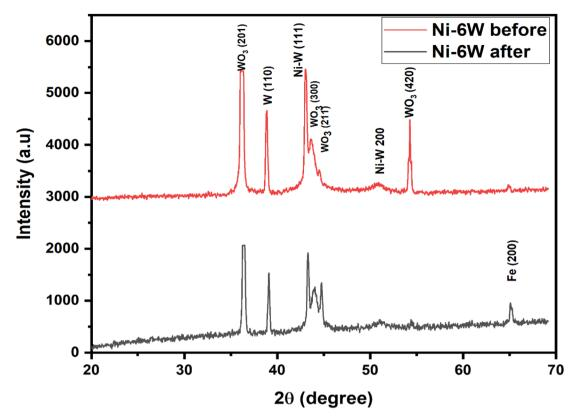
Fig. 10 XRD patterns of electrodeposited Ni-6W alloy before and after stability test.
