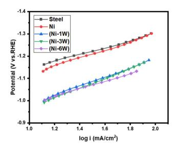
Fig. 5 Tafel plots of hydrogen evolution reaction on the deposited electrocatalytic materials in 1 mol  $L^{-1}$  KOH at 298 K.
