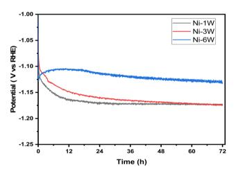
Fig. 6 Chronopotentiometric curves for HER on the surface of Ni–1W, Ni–3W, and Ni–6W coatings at a current density of  $-50~\rm mA~cm^{-2}$ .
