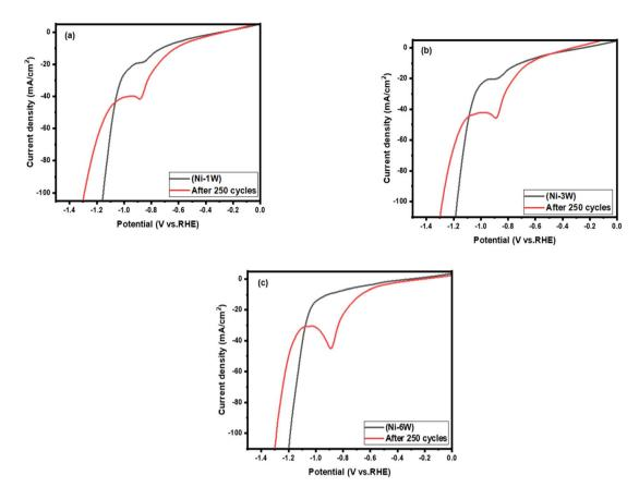
Fig. 7 LSV for (a) Ni-1W, fresh and after 250 cycles; (b) Ni-3W, fresh and after 250 cycles; and (c) Ni-6W, fresh and after 250 cycles. The curves are collected in 1 mol L<sup>-1</sup> KOH at 298 K with a scan rate of 50 mV s<sup>-1</sup>.
