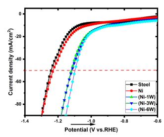
Fig. 4 Polarization curves of the HER on the deposited electrocatalytic materials in 1 mol  $\rm L^{-1}$  KOH at 298 K. The potential scan rate is 50 mV s<sup>-1</sup>.
