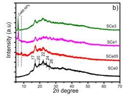
Fig. 6 TGA (a) and XRD patterns (b) of SCex Films.
