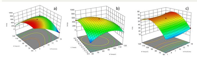
Fig. 1 3D surface plots illustrating the effects of various factors on the surface area of Ce66 NPs: (a) temperature and FA; (b) temperature and time on the surface area and (c) temperature and FA on the yield of Ce66 NPs.
