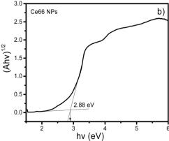
Fig. 4 UV\_Vis DRS (a) and  $E_{\rm bg}$  (b) of Ce66 NPs.
