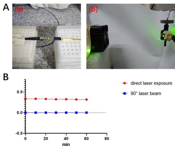
**Fig. 2** (A) (a) The laser is connected to the optical fiber and then directly irradiates the silicon phototube (b) schematic diagram of the silicon phototube receiving the emitted light at 90° to the excitation light. (B) Continuous irradiation of the laser for 60 min with continuous voltage changes at different angles.
