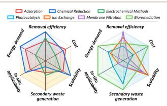
Fig. 6 Comparative analysis of the main  $Cr(v_i)$  remediation technologies using radar charts. The axes for cost, energy demand, and secondary waste generation are on an inverted scale, where a higher value represents lower value.
