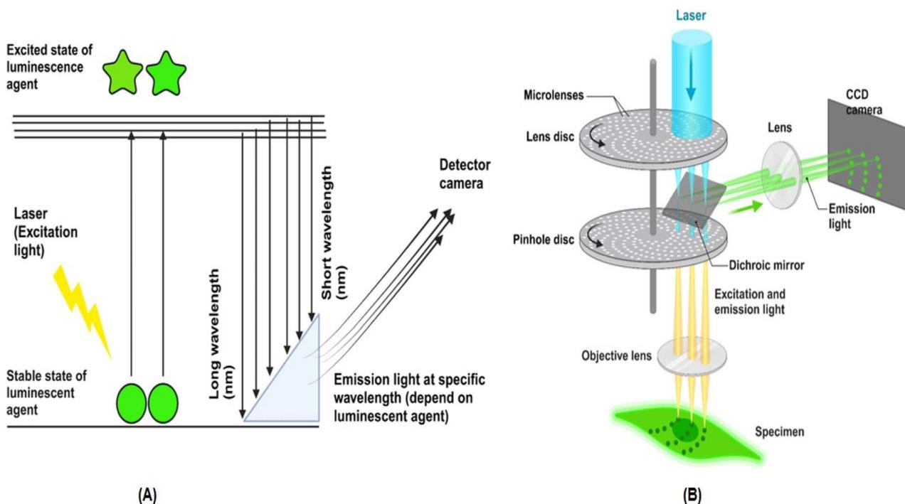
Fig. 1 Principle of FI using luminescence agent such as green fluorescence probe (GFP) and confocal microscopy. (A), a schematic of principles of FMI, (B), fluorescence confocal microscopy and various stages of FI and recording image from sample.
