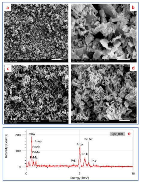
Fig. 2 (a-d) FESEM images at different magnifications; (e) EDX pattern of the prepared Pr<sub>6</sub>O<sub>11</sub> NPs.
