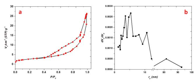
Fig. 3 BET analyses (a) adsorption-desorption (b) pore diameter of the prepared Pr<sub>6</sub>O<sub>11</sub>.
