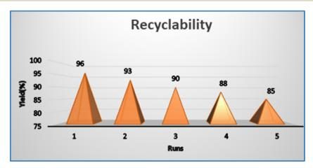
Fig. 8 Recyclability test of Pr<sub>6</sub>O<sub>11</sub> NPs.
