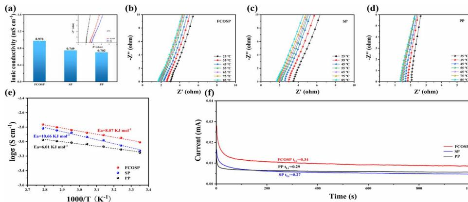
Fig. 3 Electrochemical characterization of different samples. (a) Ionic conductivity of different samples at  $25^\circ\text{C}$ , (b–d) impedance spectra of symmetric cells with different samples at various temperatures, (e) Arrhenius plots corresponding to the impedance data of different samples, (f)  $i-t$  curves of Li/Li symmetric cells with different samples at  $10 \text{ mV}$ .
