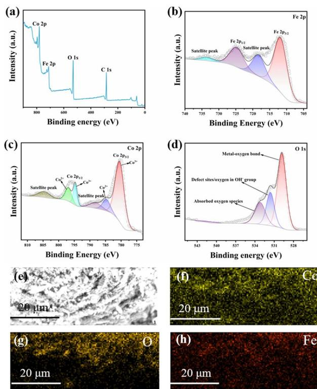
Fig. 1 Characterization of  $\text{FeCo}_2\text{O}_4$ . (a) XPS spectrum of  $\text{FeCo}_2\text{O}_4$ , (b) Fe 2p spectrum, (c) Co 2p spectrum, (d) O 1s spectrum, (e–h) EDS images of  $\text{FeCo}_2\text{O}_4$  and corresponding elemental distributions of Co, O, and Fe.
