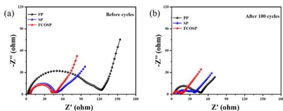
Fig. 5 Electrochemical impedance spectroscopy (EIS) of different samples. (a) Impedance spectra of different samples before 100 cycles, (b) impedance spectra of different samples after 100 cycles.
