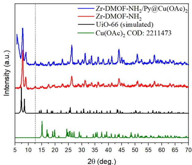
Fig. 2 XRD pattern of different stages of the synthesis of the catalyst with UiO-66 (CCDC: 2054314) and Cu(OAc)<sub>2</sub> (COD:2211473).
