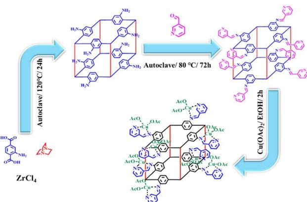
Scheme 4 Synthesis of Zr-DMOF-N/Py@Cu(OAc)<sub>2</sub> as a heterogeneous and porous catalyst.
