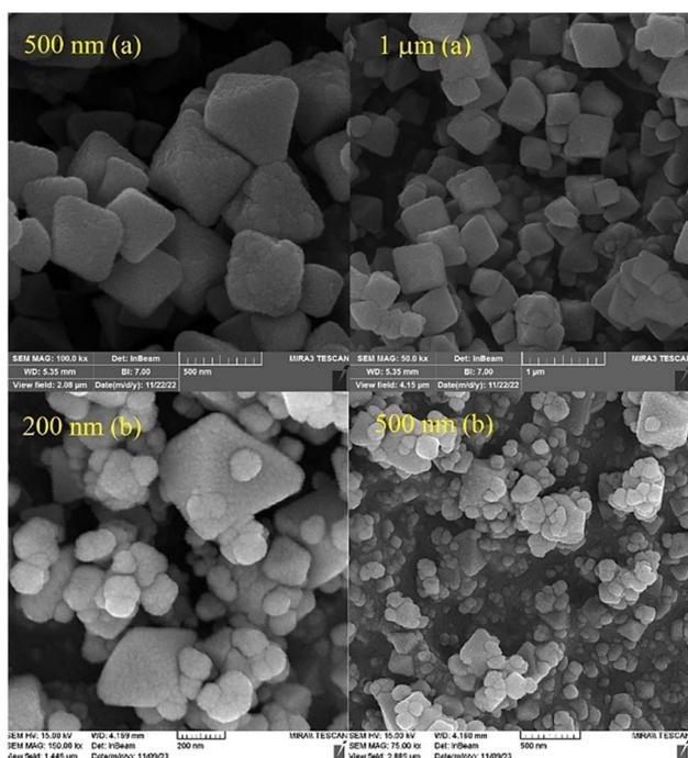
Fig. 3 SEM image of (a) Zr-DMOF-NH<sub>2</sub> and (b) Zr-DMOF-N/Py@Cu(OAc)<sub>2</sub> as a porous catalyst.
