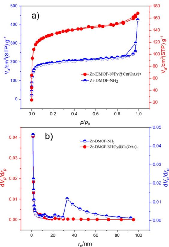
Fig. 4 (a) N<sub>2</sub> adsorption-desorption isotherms and (b) pore size distribution of Zr-DMOF-NH<sub>2</sub> and Zr-DMOF-N/Py@Cu(OAc)<sub>2</sub>.
