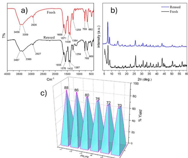
Fig. 8 (a) FT-IR and (b) XRD analysis of fresh and reused Zr-DMOF-N/Py@Cu(OAc)<sub>2</sub>. (c) Recyclability of Zr-DMOF-N/Py@Cu(OAc)<sub>2</sub> as catalyst in the synthesis of pyrazolo[3,4-*b*]pyridine derivatives.
