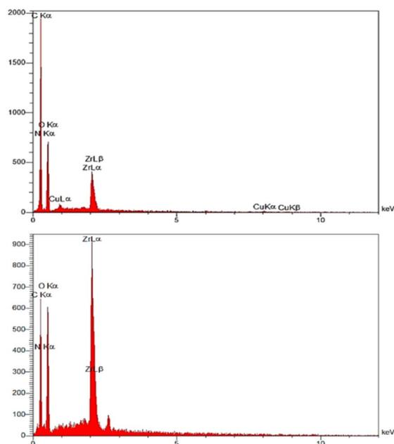
Fig. 5 Energy-dispersive X-ray spectroscopy (EDX) for Zr-DMOF-NH<sub>2</sub> and Zr-DMOF-N/Py@Cu(OAc)<sub>2</sub>.
