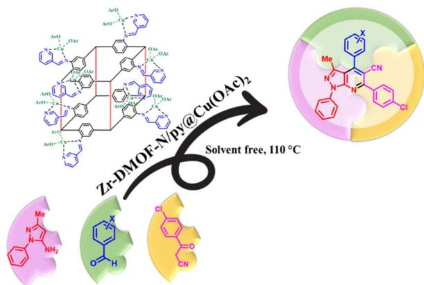
Scheme 3 Catalytic application of Zr-DMOF-N/Py@Cu(OAc)<sub>2</sub> for the preparation of pyrazolo[3,4-*b*]pyridine derivatives.
