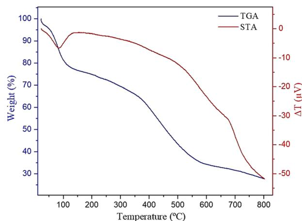
Fig. 7 TG/STA analysis of Zr-DMOF-N/Py@Cu(OAc)<sub>2</sub>.
