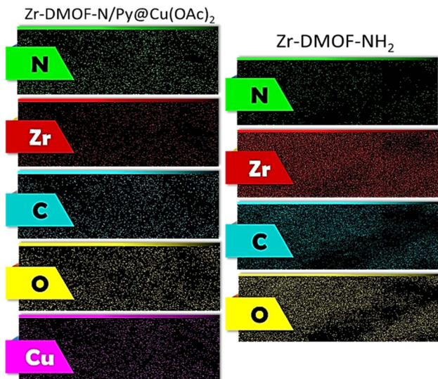
Fig. 6 Elemental mapping analysis of Zr-DMOF-NH<sub>2</sub> and Zr-DMOF-N/Py@Cu(OAc)<sub>2</sub>.
