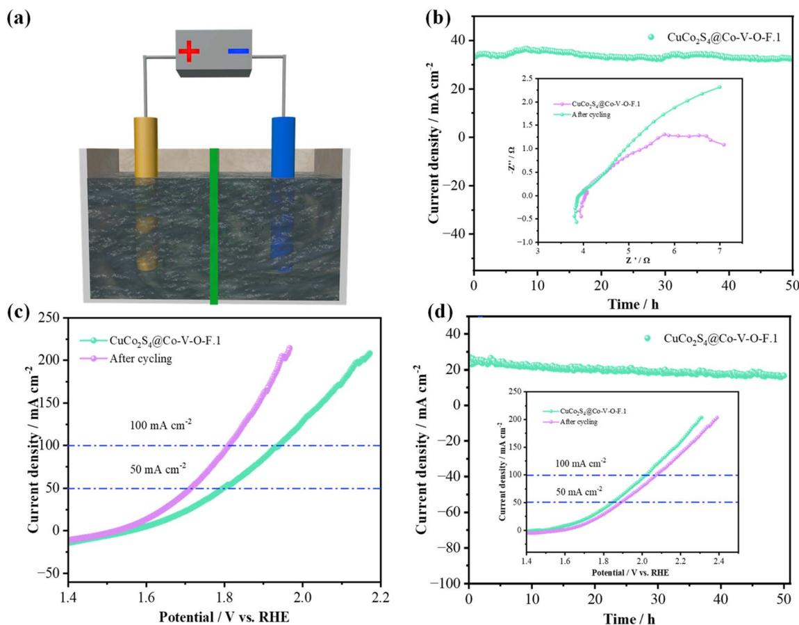
Fig. 8 Overall water splitting performance of the electrocatalysts. (a) Device schematic diagram. (b) Overall water splitting stability for  $\text{CuCo}_2\text{S}_4@\text{Co-V-O-F.1}$  in  $1.0 \text{ M KOH}$ . (c) LSV curves. (d) Chronoamperometric stability tests the insets is LSV curve in alkaline seawater.
