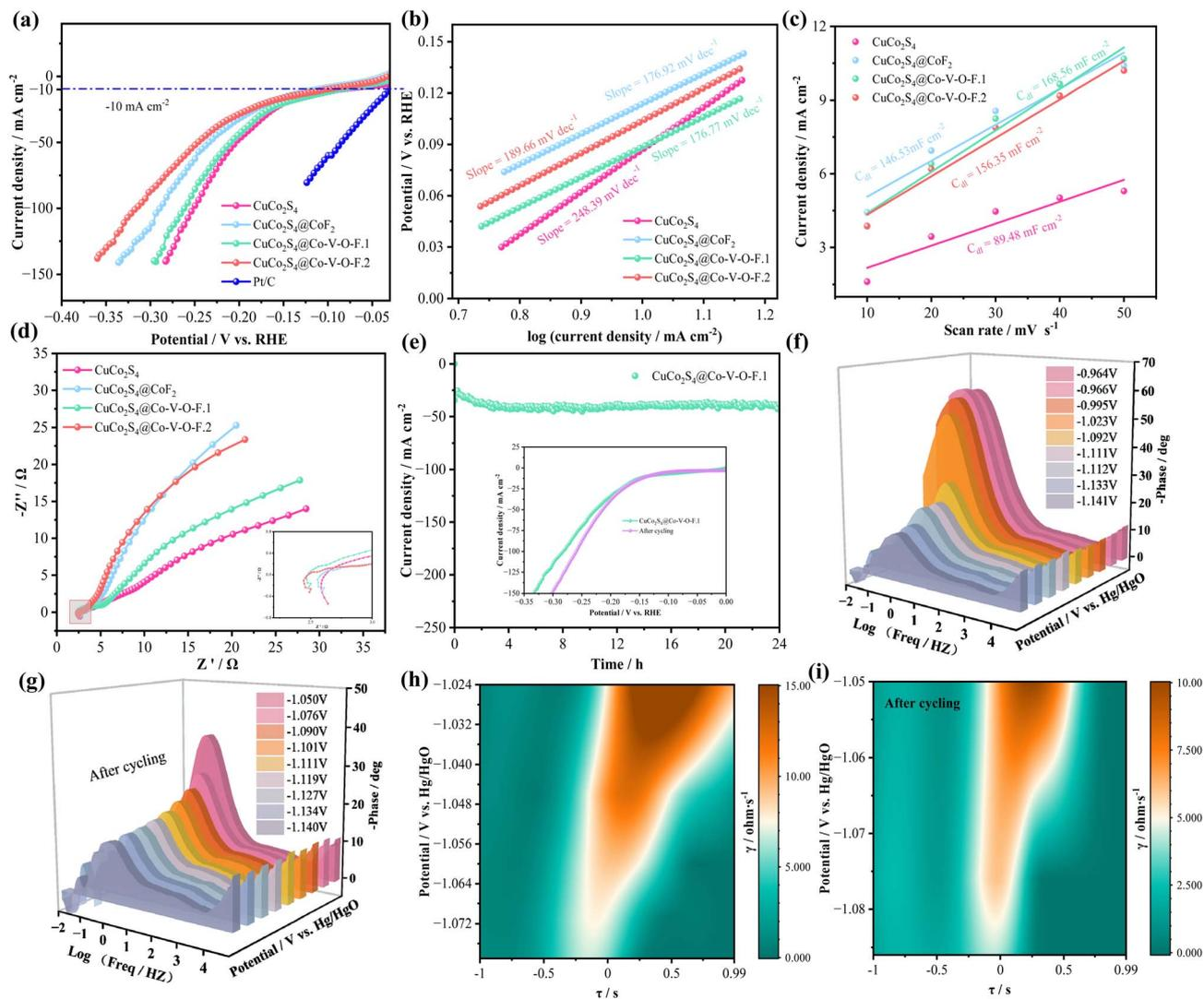
Fig. 3 HER performances in 1.0 M KOH solutions. (a) Polarization curves at scan rate of 5 mV s<sup>-1</sup>. (b) Tafel plots. (c) CV curves of double-layer capacitance ( $C_{dl}$ ). (d) Nyquist plots. (e) Chronoamperometric stability tests and the insets are LSV curves. (f and g) Nyquist plots at multiple voltages. (h and i) DRT spectrum of CuCo<sub>2</sub>S<sub>4</sub>@Co-V-O-F.1 sample before and after cycling.
