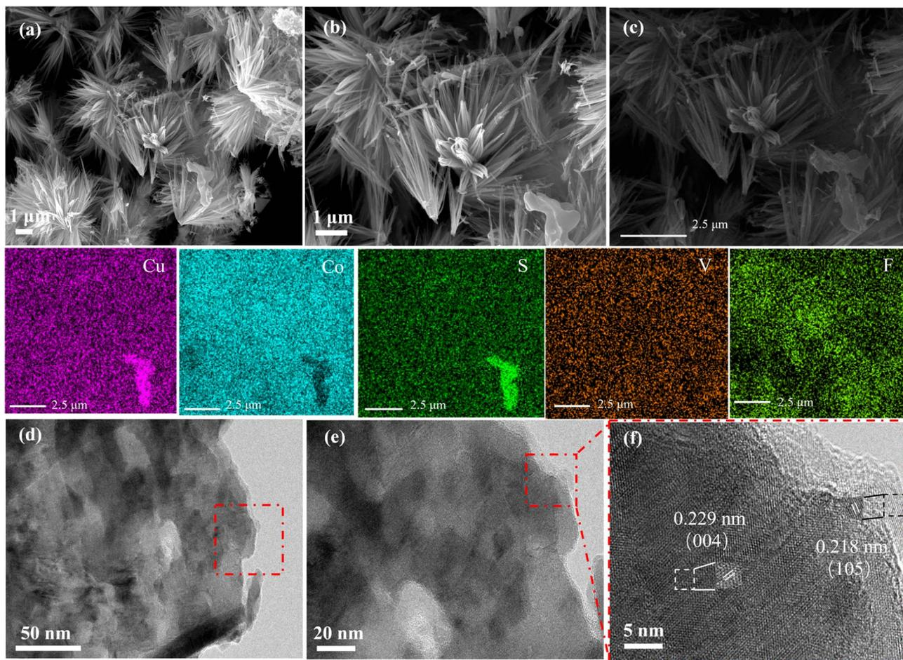
Fig. 2 Morphology and structure characterization of the as-prepared products. (a and b) SEM images of  $\text{CuCo}_2\text{S}_4@\text{Co-V-O-F.1}$  (c) EDS elemental mapping of Cu, Co, S, V and F for  $\text{CuCo}_2\text{S}_4@\text{Co-V-O-F.1}$ . (d and e) TEM images of  $\text{CuCo}_2\text{S}_4@\text{Co-V-O-F.1}$  samples. (f) HRTEM image of the  $\text{CuCo}_2\text{S}_4@\text{Co-V-O-F.1}$  composite.
