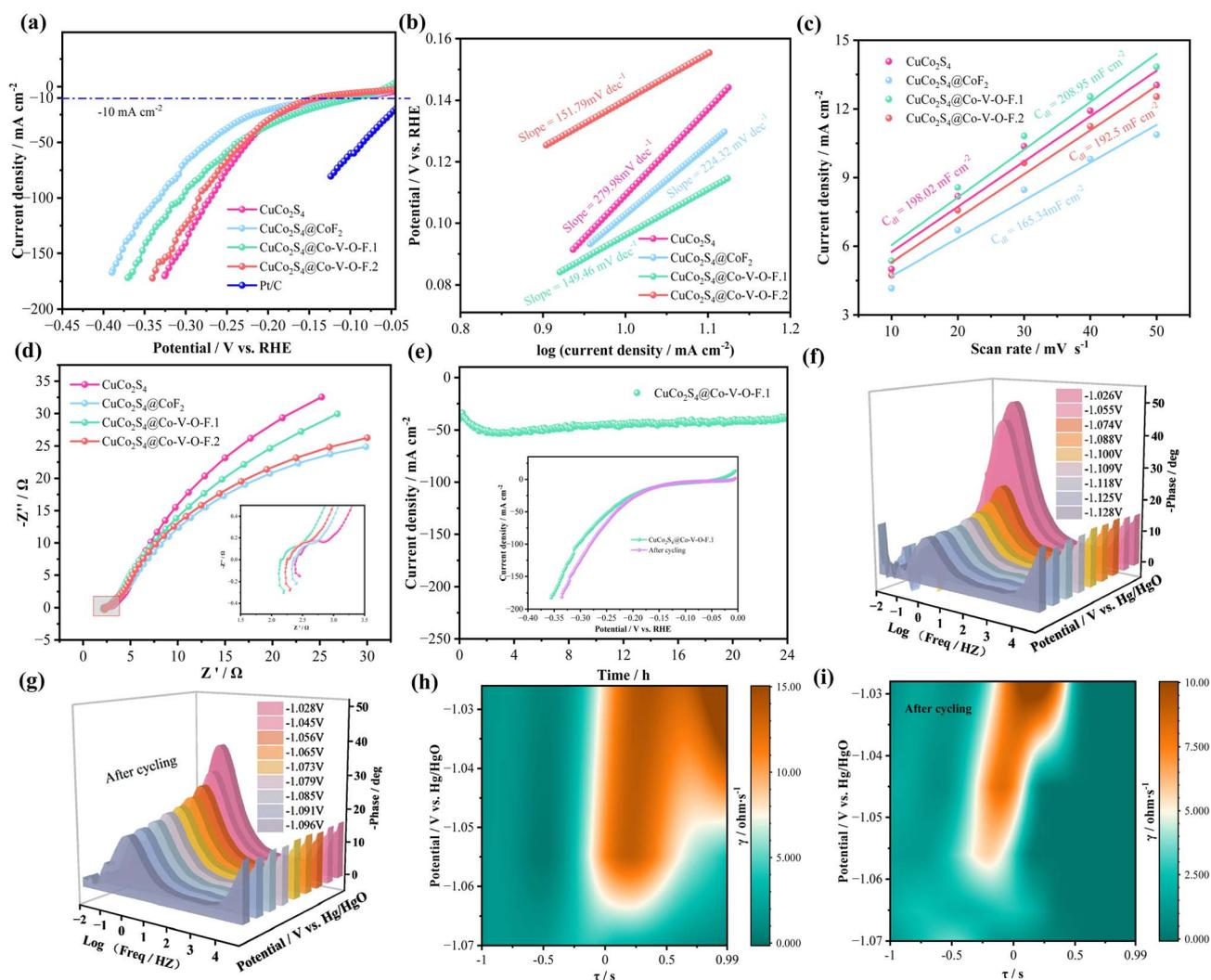
Fig. 6 Electrochemical performances of the electrocatalysts in alkaline seawater. (a) LSV curves for HER. (b) Tafel plots. (c) Double-layer capacitance ( $C_{dl}$ ). (d) Nyquist plots. (e) Chronoamperometric stability tests and the insets are LSV curves. (f and g) Nyquist plots at multiple voltages. (h and i) DRT spectrum of  $\text{CuCo}_2\text{S}_4@Co-V-O-F.1$  sample before and after cycling.
