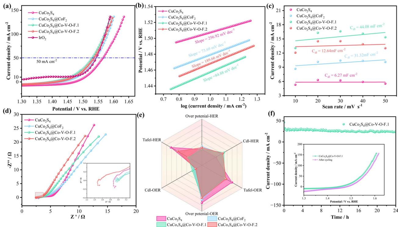
Fig. 4 OER performances in 1.0 M KOH solutions. (a) Polarization curves at scan rate of 2 mV s<sup>-1</sup>. (b) Tafel plots. (c) Double-layer capacitance (C<sub>dl</sub>). (d) Nyquist plots. (e) Radar chart. (f) Chronoamperometric stability tests the insets are LSV curves before and after cycling.
