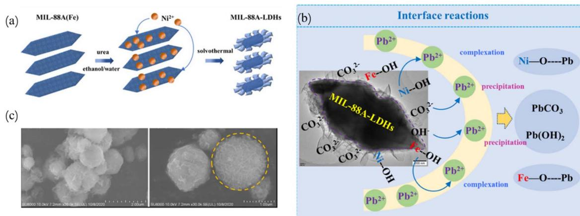
Fig. 3 Schematic illustration of the synthesis process of MIL-88A-LDHs (a). Schematic illustration of the mechanism of  $\text{Pb}^{2+}$  adsorption by MIL-88A-LDHs (b). SEM images of MIL-88A-LDHs (c). Reprinted with permission from ref. 93. Copyright (2022), MDPI.
