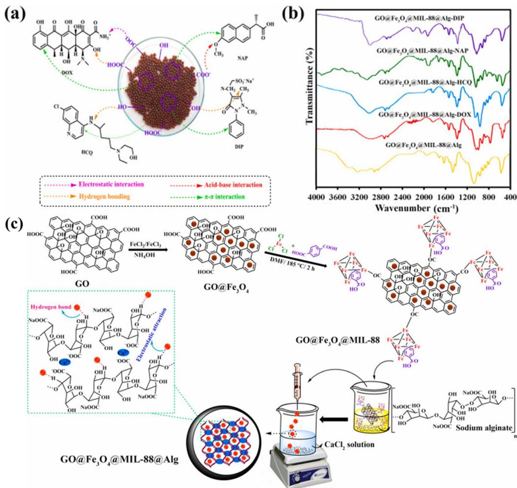
Fig. 4 Proposed adsorption mechanism of DOX, HCQ, NAP, and DIP onto GO@Fe<sub>3</sub>O<sub>4</sub>@MIL-88@Alg hydrogel beads. (a) FT-IR analyses of GO@Fe<sub>3</sub>O<sub>4</sub>@MIL-88@Alg hydrogel beads post-adsorption of DOX, HCQ, NAP, and DIP. (b) Schematic of sequential steps for removal of COVID-19 drugs using GO@Fe<sub>3</sub>O<sub>4</sub>@MIL-88@Alg hydrogel beads. (c) Reprinted with permission from ref. 99. Copyright (2024), Elsevier.
