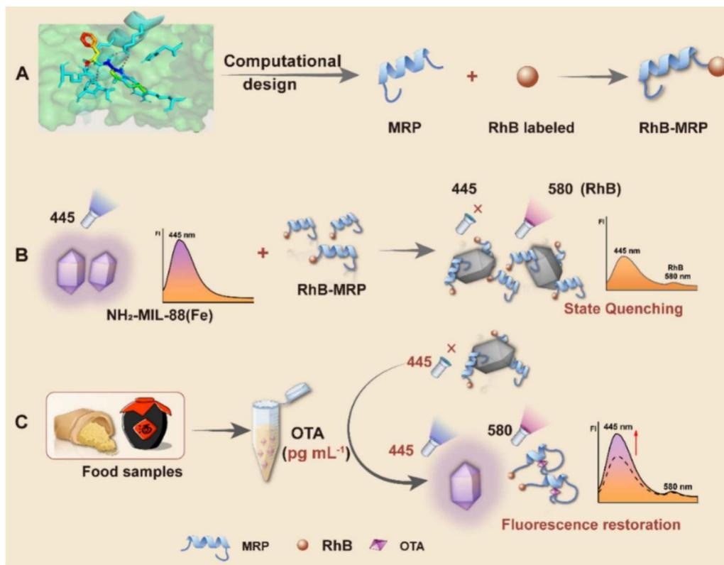
Fig. 6 Schematic diagram for the construction of fluorescence biosensor based on RhB-MRP and NH<sub>2</sub>-MIL-88(Fe). (A) Design of MRP and Pep-RhB. (B) Synthesis of NH<sub>2</sub>-MIL-88(Fe) and its fluorescence quenching upon interaction with RhB-MRP. (C) Fluorescence recovery of NH<sub>2</sub>-MIL-88(Fe) upon addition of OTA. Reprinted with permission from ref. 152. Copyright (2025), Elsevier.
