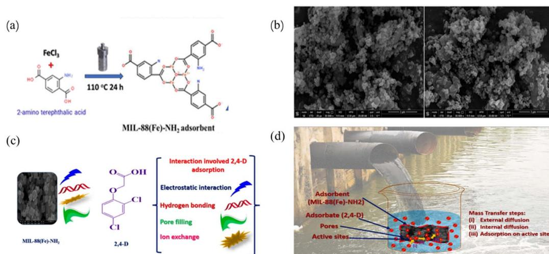
Fig. 5 Hydrothermal synthesis of MIL-88(Fe)-NH<sub>2</sub>. (a) SEM images of MIL-88(Fe)-NH<sub>2</sub>: before adsorption (left) and after five reuse cycles (right). (b) Interaction mechanism between MIL-88(Fe)-NH<sub>2</sub> adsorbent and 2,4-dichlorophenylacetic acid molecule. (c) Diffusion mechanism of 2,4-dichlorophenylacetic acid onto MIL-88(Fe)-NH<sub>2</sub>. (d) Reprinted with permission from ref. 101. Copyright (2023), ACS.
